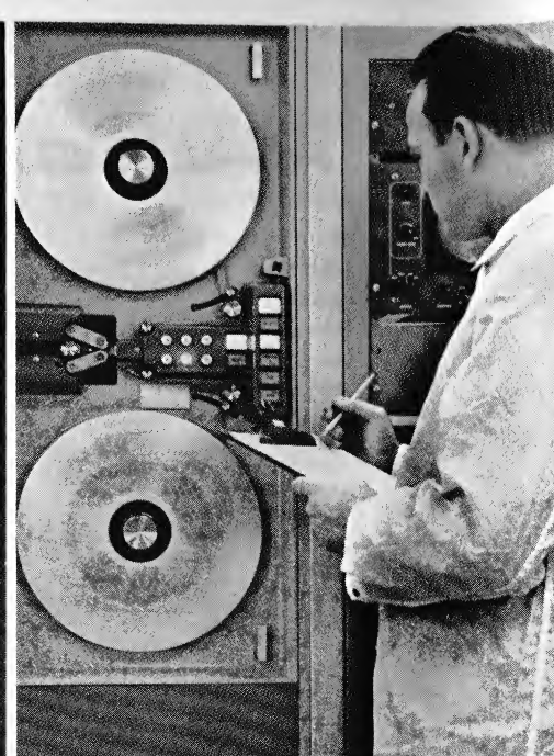
Dropout and wear tests (above) literally run tapes "to death" to determine the effective life of a sample. Tapes with low dropouts, not only on the first pass but also on the 100th pass and far beyond, are vital in many present-day applications. This Audio engineer (below) is testing the physical properties of tapes under unusual conditions which may be encountered in space vehicles.
