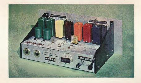
An illustration in the use of the model 70 series module is the new Stancil-Hoffman ARP-70 mixer-recordplayback unit. From left to right are two AL-70 microphone preamplifiers, the AP-70 preamplifier, the AH-70H line amplifier, AR-70 record amplifier, AO-70 bias oscillator and the AW-70L monitor amplifier which feeds a built-in speaker.
