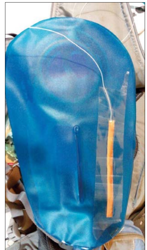
Figure 5. The DIY sensor works equally well when mounted at the other side of the reservoir.
