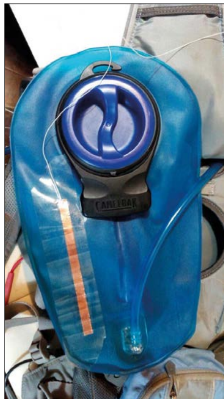
Figure 4. The water reservoir with the capacitive sensor secured to it. Oh yes, these reservoirs can be bought at hiking and outdoor outlets.
