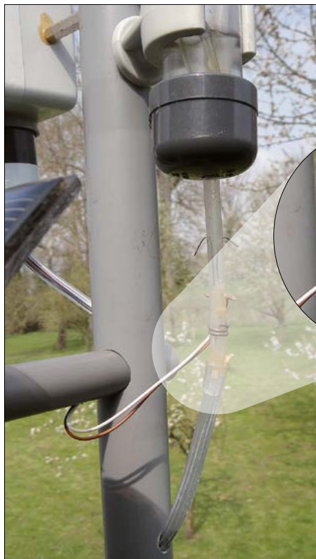
Figure 3. These are the two electrodes at the siphon outlet that detect the emptying.
