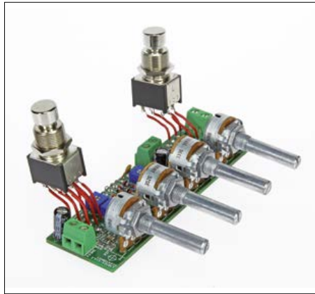
Figure 3. With this prototype you can clearly see how the switches are connected.
