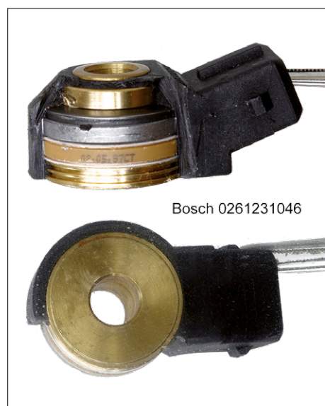
Figure 1. The knock sensor consists of a disc made out of a piezo-electric material, which has been sandwiched between a couple of metal discs.
