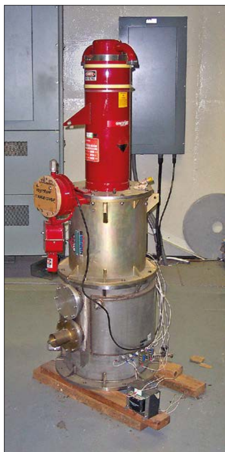
Figure 2. Klystron. Source: Enoch Lau at English Wikipedia.
