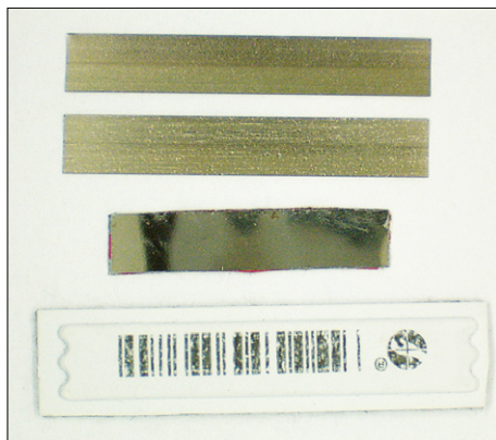
Figure 1. The AM label components, shown here are two resonators and a (shorter) magnetic strip.
