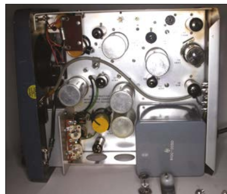
Figure 5. Cleaned chassis with V9 broken off at the base.
