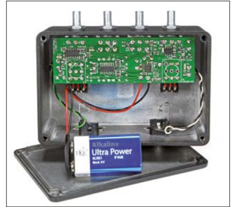
Figure 4. This is how the circuit is mounted into a sturdy enclosure.
