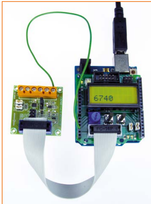
Figure 4. To test the ADC module and the Data logger application connect a wire from the Arduino pin A3 to the ADC input at AIN0.
