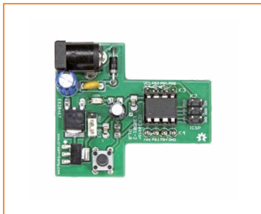
Figure 4. T-Board 8 prototype. Small differences may exist with the final version supplied through the Elektor Store.
