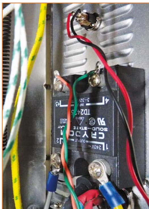
Figure 8c. Detail of the salvaged solid-state relay and the 5 V socket.
