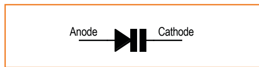
Figure 1. Varactor (varicap) schematic symbol.
