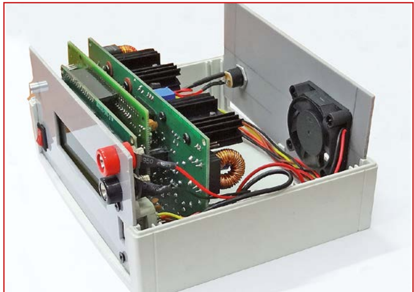
Figure 3. Looking inside the enclosure from the right. The three boards that make up the little supply (LCD, Platino, PSU) are fitted vertically behind the front panel.
