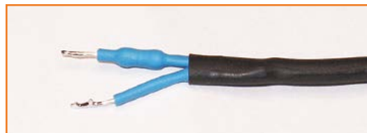
Figure 5. The DIY low-impedance probe.
