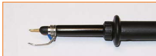
Figure 4. A standard Hameg probe with DIY tip-ground modification. The Earth lead is removed.
