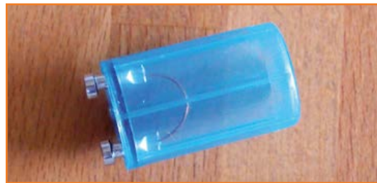
Figure 3. The starter supplied with the LED lamp is just a wire link.
