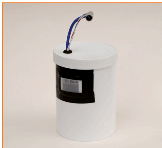
Figure 6. The entire circuit housed in a splash-proof enclosure.
