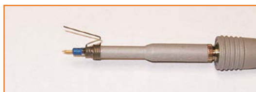
Figure 2. An Agilent probe with the Earth lead removed, using a ground spring.
