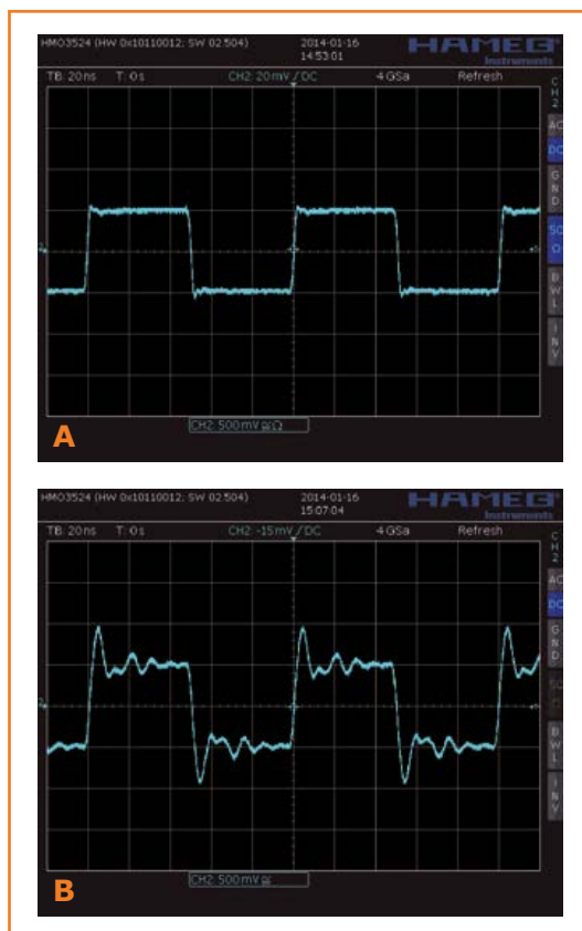
Figure 1. 10-MHz square wave signal using coax and 50-Ω termination at the scope input (A); The same signal measured with a standard probe and a flying Earth lead (B).
