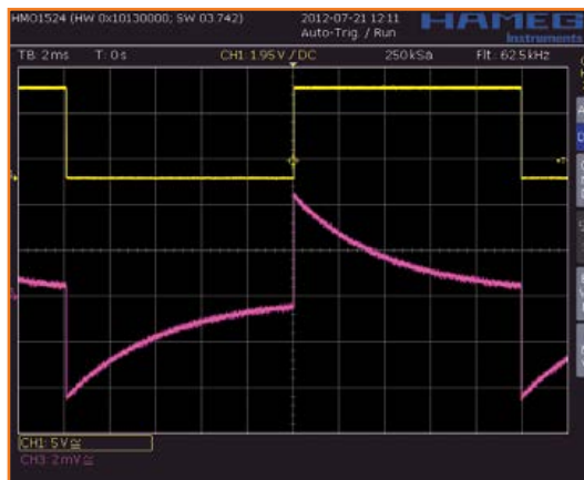
Figure 3. Measuring a 50 Hz square-wave signal with a ferrite ring.
