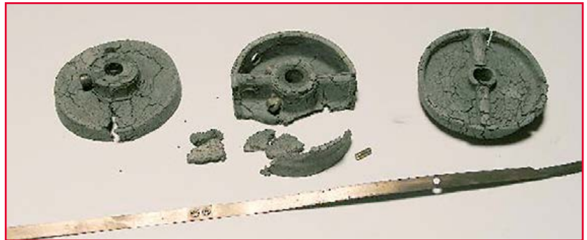
Figure 4. Disintegrated pulleys: photograph reproduced with permission of Allen Wooten, WD4EUI.
