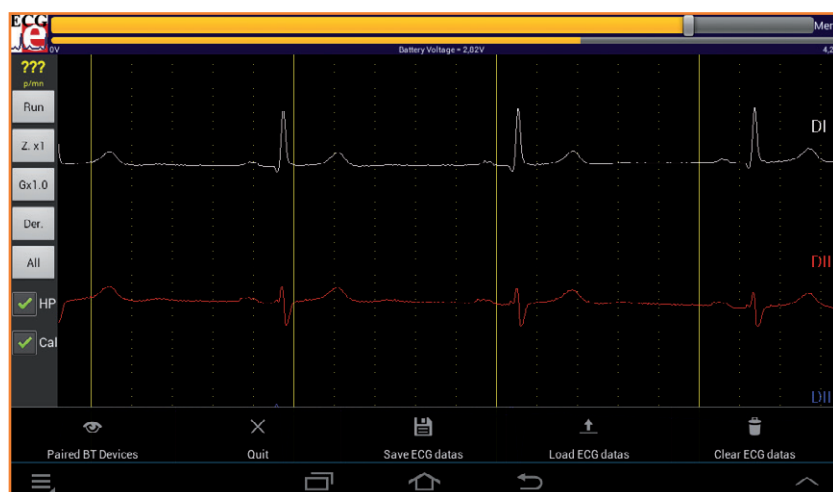
Figure 15. The menu functions: BT connection, quit, saver and load ECGs, erase ECG memory.
