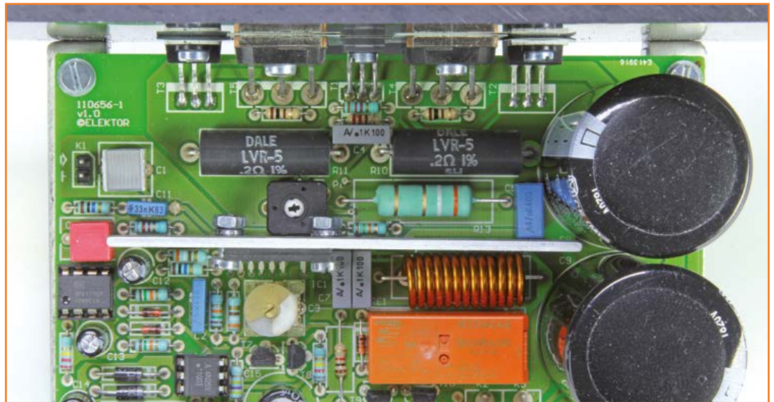
Figure 5. There's just enough space on the circuit board for the heatsink that has to be mounted on IC1.
