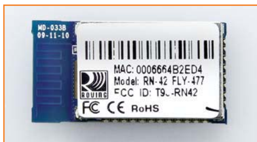
Figure 4c. Photo of the Roving Networks (now Microchip) Bluetooth module used.
