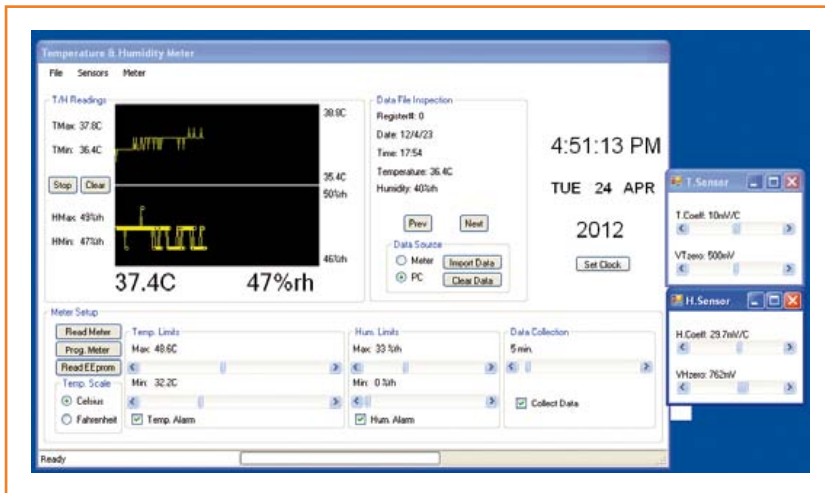
Figure 3. The Graphical User Interface allows easy access to the various settings of the Temperature & Humidity Meter.
