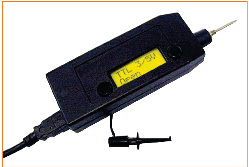
Figure 1. The multitester design by Thomas Ücok is based on the Elektor Minimod module.
