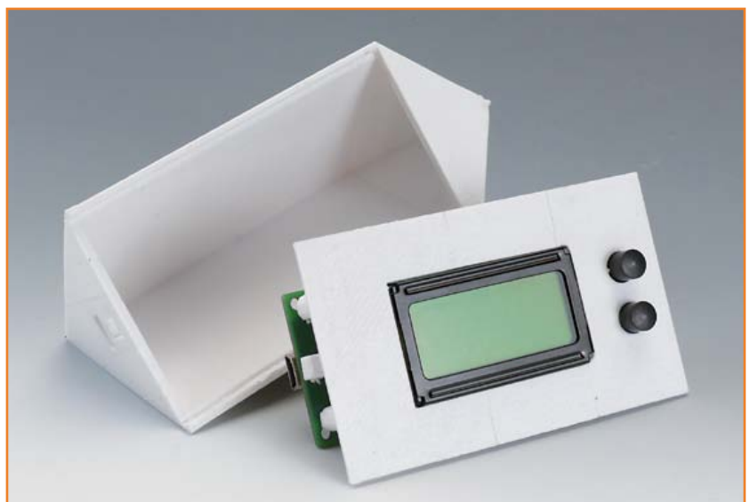
Figure 2. An enclosure for the project can be made using a 3D printer.
