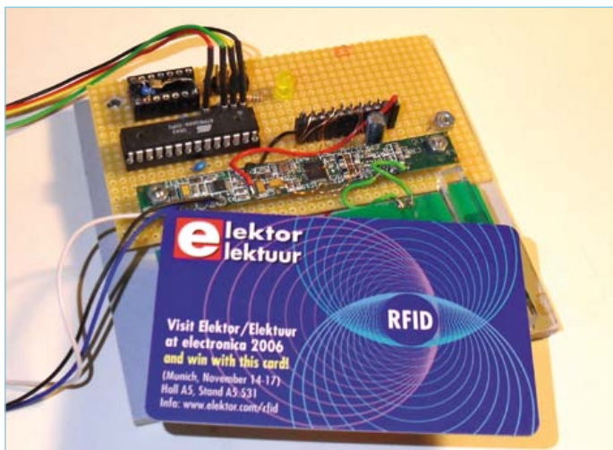
Figure 4. Prototype with ATmega88 and PN512 reader board.
