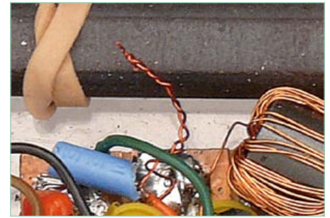
Figure 5. C7 is formed by two wires twisted together – a 'pigtail' capacitor.
