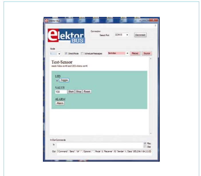
Figure 7. The PC program simulates an external instrument or sensor.
