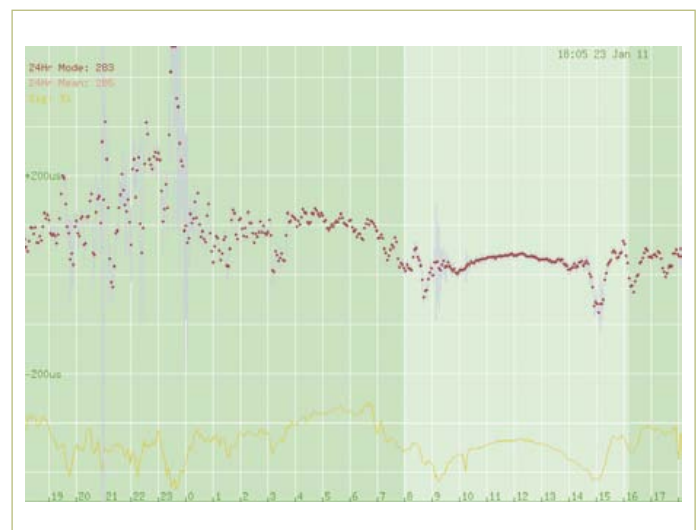
Figure 6. DCF77 receiver typical short-term (24 hour) performance. Red dots show average timing accuracy over a 200 s period with grey lines indicating stanrad deviation over that period. Vertical axis is 100 \mu\text{s} per division. Ideal performance would be a flat line across the centre. The yellow line indicates signal strength. Notice the contrast between day-time (10 am - 2 pm) and night-time performance.
