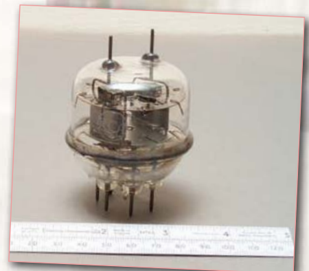
The 832-A twin tetrode transmitting tube. An old time favourite among radio hams. No neutrodynization as opposed to the European QQE06/40 (see also Retronics December 2008).
