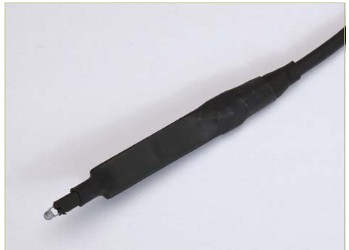
Figure 1. The sensor board inside the temperature probe supplies a serial digital output signal.
