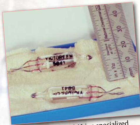
The Victoreen 5841 is a specialized subminiature high-voltage gas regulator tube. It regulates at 900 VDC for a load of 5-100 \mu A.
