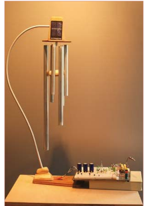
Figure 3. The chime sounds when enough energy has been harvested. This saves watching the meter all the time.
