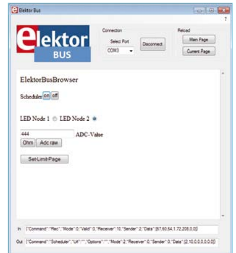
Figure 1. Screenshot of the first version of the ElektorBus browser with example application running.
