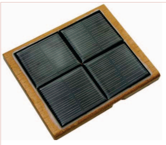
Figure 7. Solar module arrangement in the author's prototype charger.
