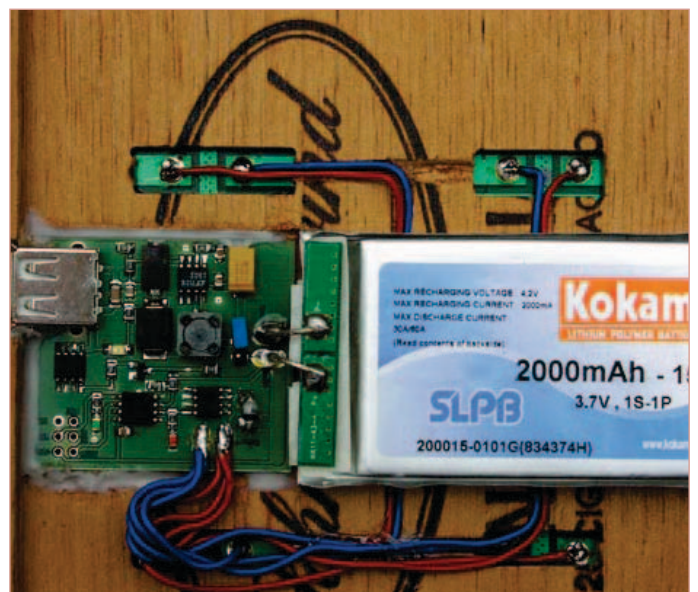
Figure 8. Internal view of the first prototype. The PCB is connected directly to the solar modules here.
