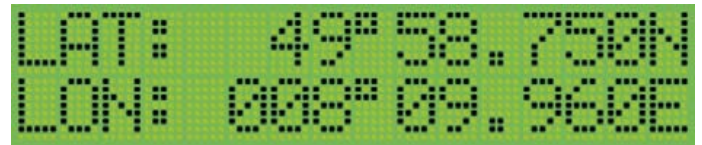
Figure 7. The display shows the GPS coordinates when switch S2 is closed.
