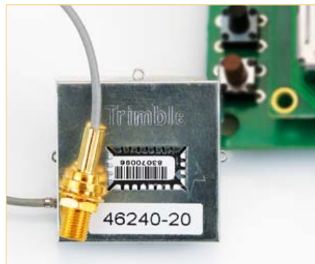
Figure 5. The lab prototype uses a GPS receiver from Trimble.
