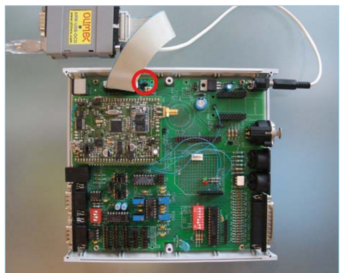
Our Sceptre / InterSceptre system. Remember to fit JP7 on the InterSceptre to enable the JTAG port.
