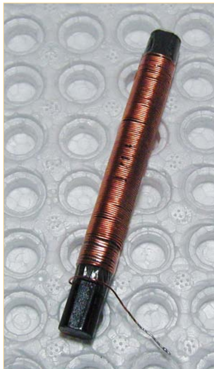
Figure 5. A radio ferrite rod makes a good core for winding a 60-160 \mu H adjustable inductor that enables the largely capacitive transducers to be peaked at their resonant frequency (usually, 40 kHz).
