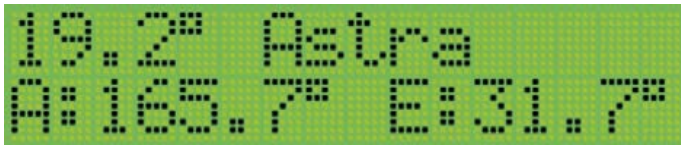
Figure 6. As soon as the GPS receiver sends positional data the azimuth and elevation of the chosen TV satellite is shown on the display.
