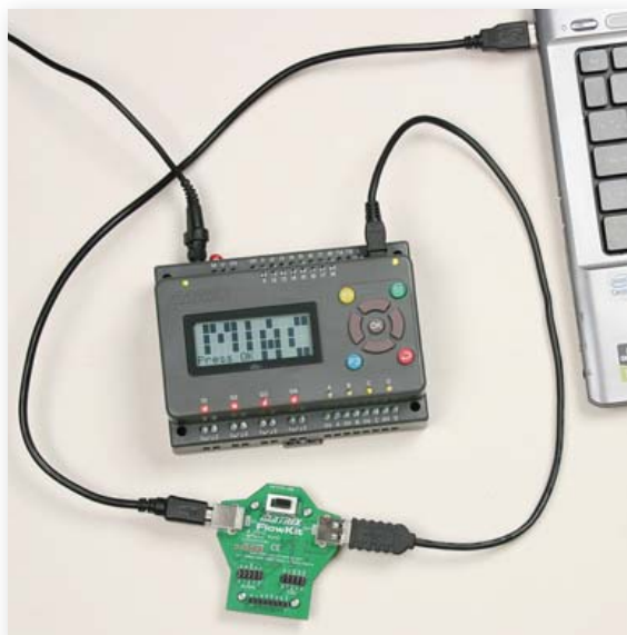
Using MIAC with FlowKit to give full IN-Circuit Debug with Flowcode
