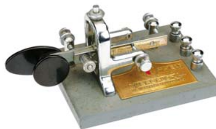
Figure 5. A collector's item and a QRQ delight, this vintage Vibroplex paddle keyer is easy to adjust to your personal preferences and rock solid on its cast iron base. Courtesy Anton Klok PA3AQV.
