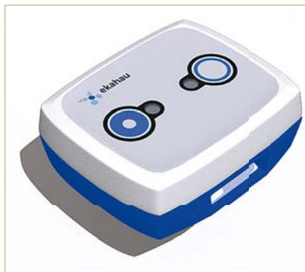
Figure 6. This RTLS Wi-Fi tag (802.11 b/g/n) attached to an object makes it possible to locate it with a range of around 50 m (150 ft.) indoors and up to 150 m (450 ft.) in free field.
