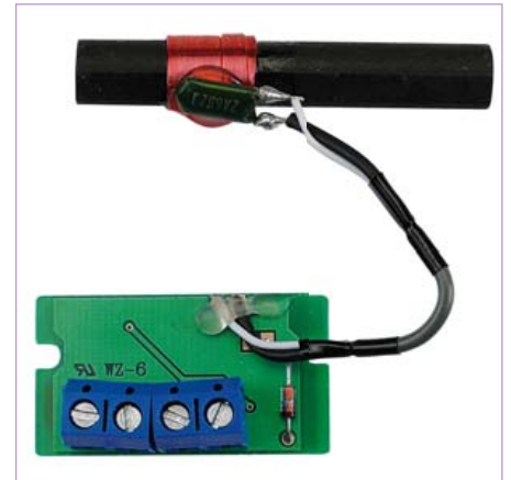
Figure 3. A DCF77 receiver module is used for precise time synchronisation. This module is based on the proven Temic DCF77 receiver IC.
