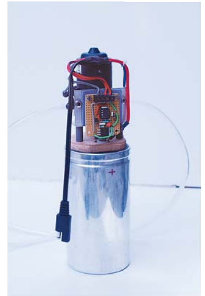
Figure 7. The circuit of Figure 6 implemented with an IRF3708 and a 0.15-MF electrolytic capacitor drives the small pump at the rear. The connector is for the solar panel.
