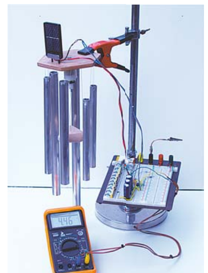
Figure 9. A solar cell supplies 0.2 to 1 V to a Dickson charge pump with 17 stages constructed on a piece of prototyping board. The motor starts running at approximately 5 V.
