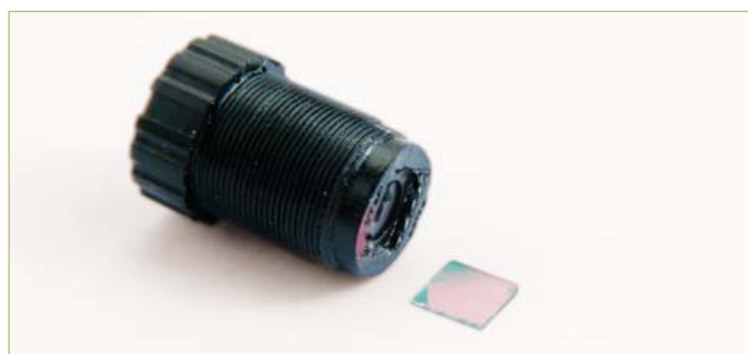
Figure 3. With the König lens the removal of the IR filter was quite easy to do.
