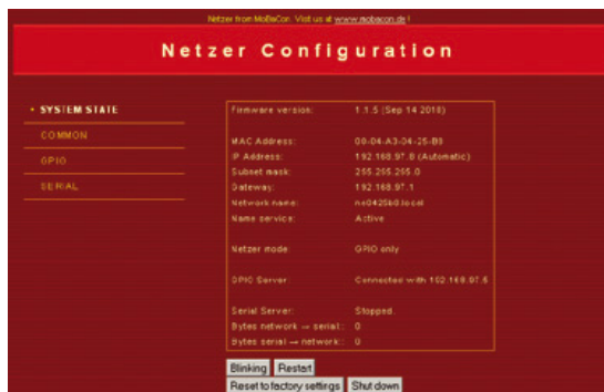
Figure 5. The home page for the module’s web interface. The ‘Blinking’ button comes in useful when more than one module is used simultaneously.
