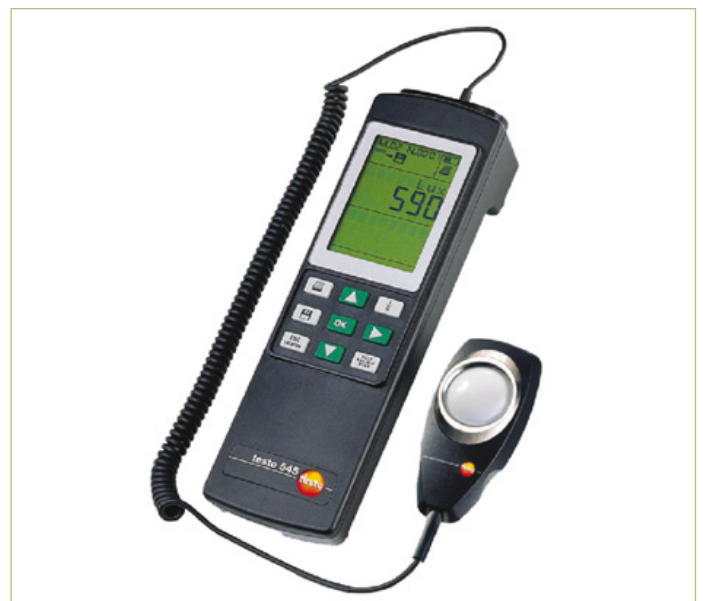
Figure 3. A lux meter measures the amount of incident light across a hemisphere. (photo: Testo).
