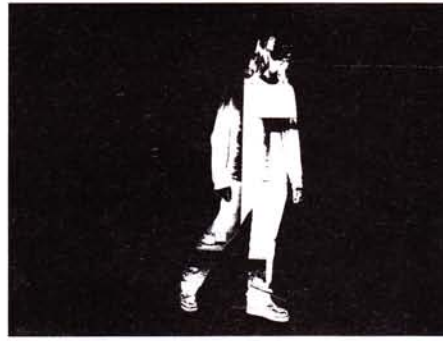
Figure 4. The result of the next step: the pixels in this image are white where the greyscale difference is greater than a defined threshold.
