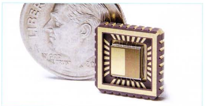
Figure 11. The SensorChip-CO 2 is a MEMS chip for measuring CO 2 (photo: ICX Technologies).
