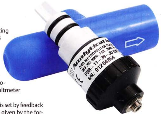
Bild 1. Sensor with adapter for connecting to a diver's breathing kit.
