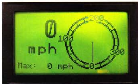
Figure 6. If the data is correct a speed display appears in km/h. Pressing S2 will switch to miles per hour (mph) which is the norm around Rocklin, CA.
