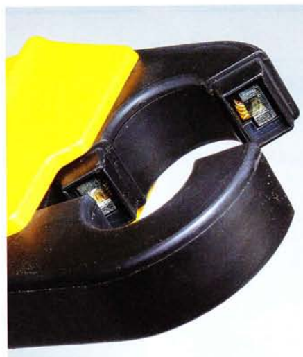
Figure 2. A pair of Hall sensors are clearly visible in the air gaps between the jaws of this Fluke clamp meter.
