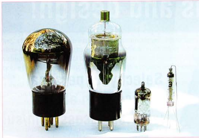
Figure 1. Eighty years back in time. Left to right: tubes type RES164, 34, EF97 and 1j18b.
