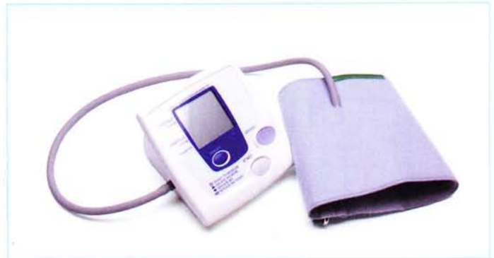
Figure 7. This blood pressure monitor can be read out remotely over a Zigbee link.
