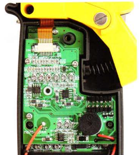
Figure 4. Clamp meters are complex instruments with many adjustment points. We counted around 15 trimpots in this model.
