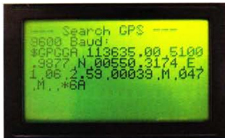
Figure 5. Switching on the unit displays the GPS Search Image based on data received at 9600 baud.
