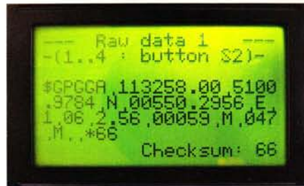
Figure 9. Display of raw GPS data. Data blocks can be called up individually.
