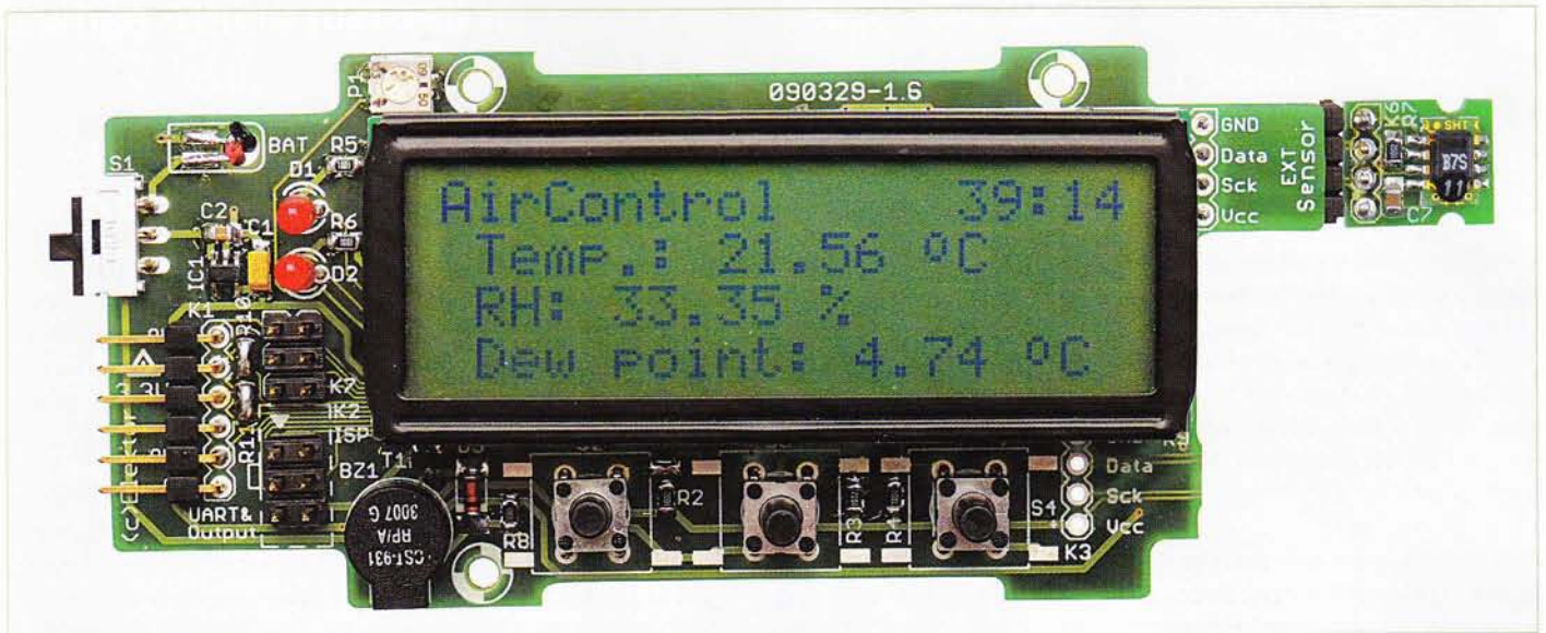
Figure 1. The PCB and main components. The great shy microcontroller is hiding under the display.
