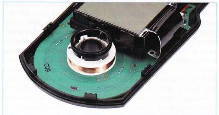
Figure 2. The Bosch and Skil pipe and wire locators use a coil facing the wall for accurate detection of metal objects. The PCB tracks around the coil form the plates of a capacitive sensor for wood detection.
