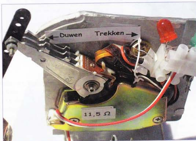
Figure 1. It makes it easier if we remove part of the aluminium plate (left) and connect the actuator coil to a terminal block (right).
