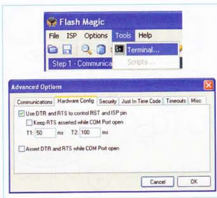
Figure 3. Here's how to run the Flash Magic terminal and configure it. The speed of the terminal's serial port can be different from that of the programming mode.
