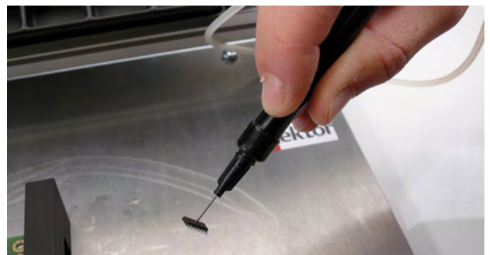
To pick and hold a component, just attach the pickup needle to the component's surface and turn on vacuum by putting your finger top on the pickup holder's side hole.
