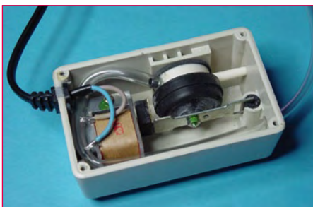
Figure 9. Pump with suction tube fitted.
