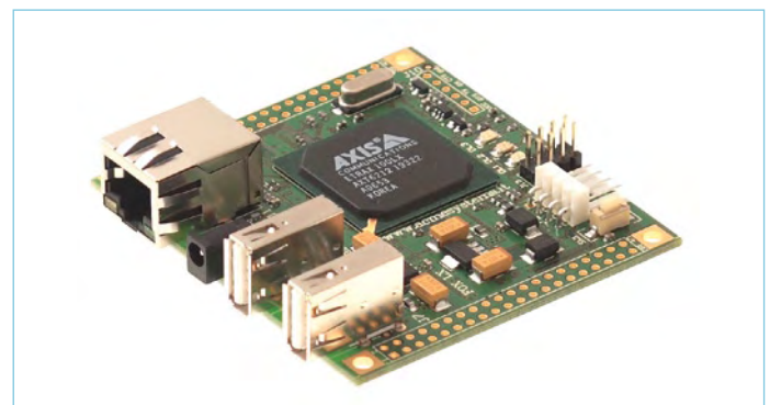
Figure 9. The FOX LX832 card by Acme Systems; This card measuring 66 × 72 mm has an Ethernet port, two USB 1.1 ports, digital I/Os, an I 2 C port, serial and parallel ports, operates under Linux and costs around $200.
