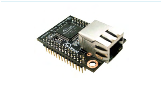
Figure 5. The WIZ 830MJ module comprises not only an Ethernet controller, but also a hardware TCP/IP stack.
