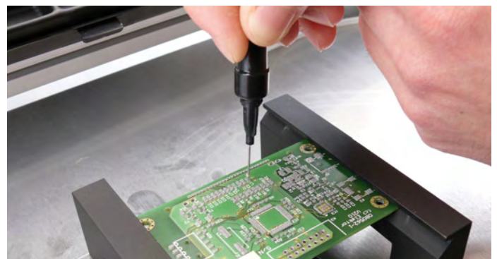
Carefully place each component on its PCB pads. To release the component, turn off the vacuum by removing your finger from the side hole.
