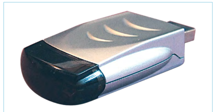
Figure 8. An IrDA USB key of unknown make (source Wikipedia)
