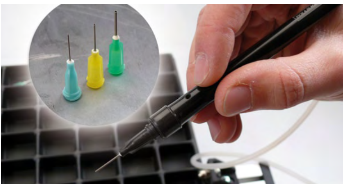
The pickup needles have different diameters to suit the size of the components handled. Connect a pickup needle to the pickup holder's nozzle and turn the pump on.
