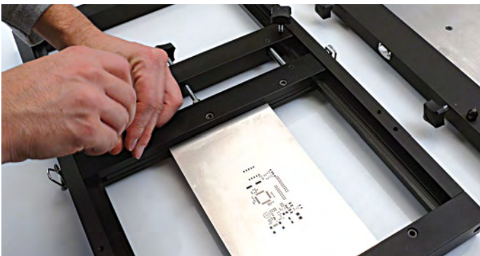
Position the stencil on the rails striving to align it with the PCB to the best of your ability. To stiffen the stencil, tighten the 6 screws using a hexagonal key. Now, close the lateral clips.
