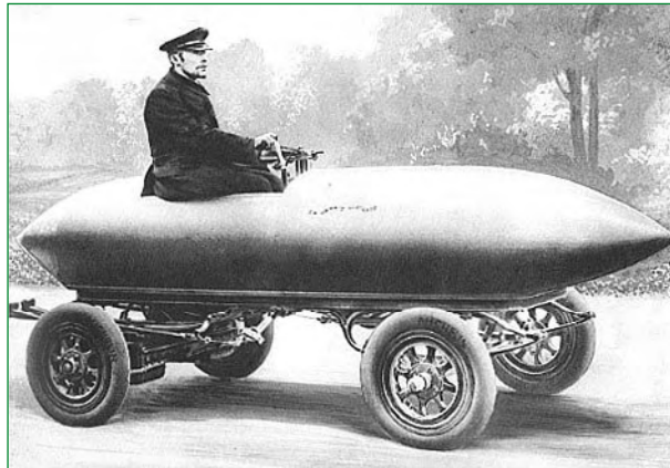
Figure 1. Back to the future: 112 years ago the electric vehicle was the leader of the pack. In 1899 Camille Jenatton reached a top speed of 105.8 km/h (66.1 mph) in a vehicle powered by lead-acid batteries delivering 50 kW.
