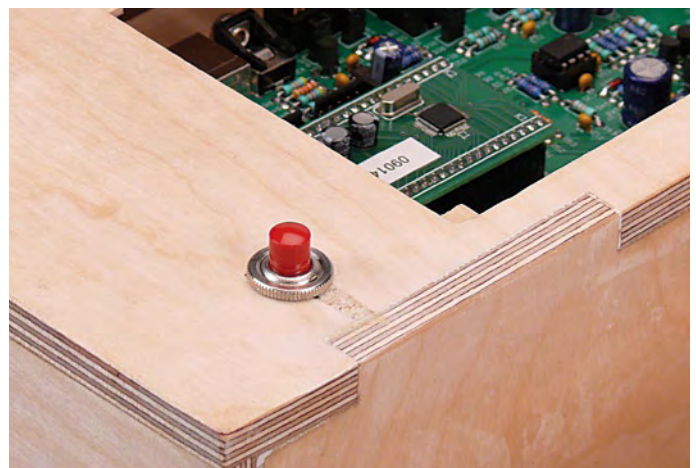
Figure 10. The emergency stop button needs to be accessible!
