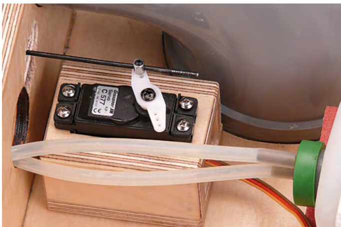
Figure 5. The throttle servo in its mount.
