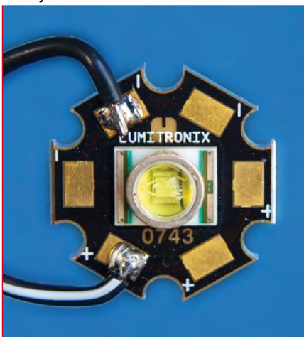
Figure 1. The 3 W LED from Cree used by the author in his experiments is a particularly beautiful piece of electronics.
