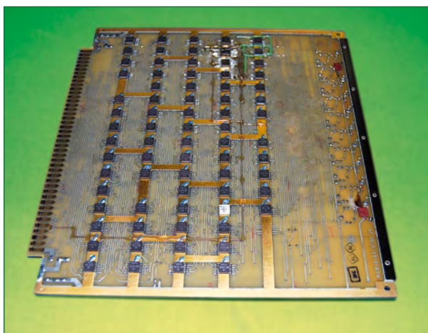
Figure 2. Flatpack logic ICs soldered to the top surface of the printed circuit board were an essential part of this 1960s mainframe computer, the most powerful of its time. The board comes from a Telefunken TR440, first produced in 1969. (Photograph: NRW Finance Authority Computer Centre, http://www.rzf-nrw.de )
