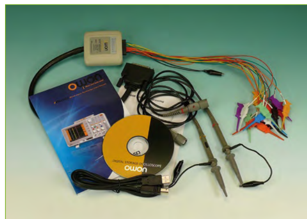
Figure 3. The package from Owon includes: Software-CD, manual, logic analyser clips, two 1:10 switchable scope probes with spares and a USB cable.
