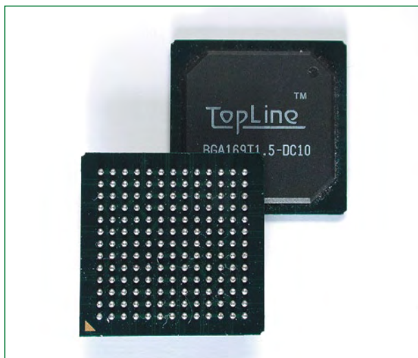
Figure 8. A device in a BGA (ball grid array) package, here with 'only' 169 solder balls.
