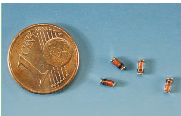
Figure 4. Diodes without wires: the cylindrical MELF package is a derivative of the leaded package.
