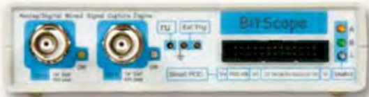
Standard 1M/20pF BNC inputs
