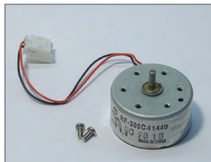
The little DC-motor as removed from the CD-drive (keep the little mounting screws).
