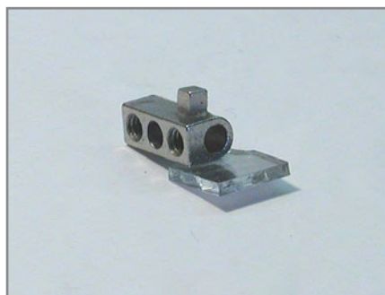
The shaft coupling with mirror and magnet, all glued together.
