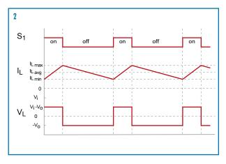
In **Figure 2** you can see the aspect of the inductor current, that is a triangle centered in the average current, rising and falling linearly when the switch is ON and OFF, respectively.
