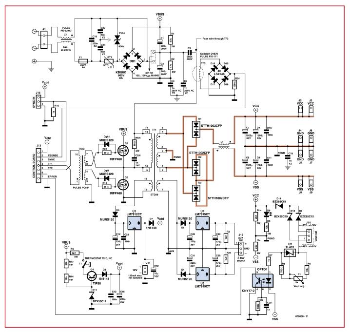
Figure 2. The circuit diagram shows the topology used, as wells as all added controls and protections.
