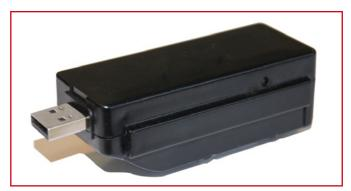
owners, as well as consumers realtime vehicle and asset tracking device that uses the immensely popular Google Earth program for high-resolution satellite imaging. Since GSM is the most prevalent mobile communications standard worldwide, the new 8100G will allow LandAirSea to expand its customer base beyond the USA and Canada.
