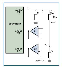
Figure 1. Block diagram for method A.
