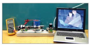
ted drive pressure to the motor (in this case 6 bar), regardless of variations in the input pressure delivered to the reservoir. The motor is naturally mechanical and coupled to a generator; with the electrical energy produced going to a DC-DC converter to produce the correct voltage for a laptop computer.
