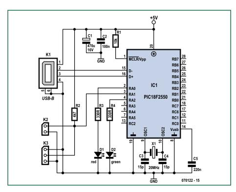
Figure 5. Circuit diagram of the Thermo-Snake central control unit. The string of DS18B20 sensors (up to 128!) is connected to K2. K3 is for learning.
