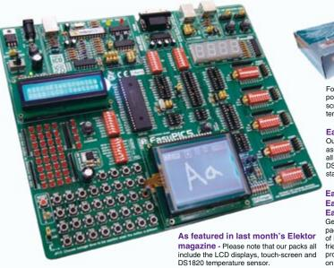
Four starter packs available, all of which include the EasyPIC5 development board, USB power/programming lead, blue backlit 16x2 character and 128x64 graphic LCDs, touchscreen overlay for GLCD, RS-232 lead, PIC16F877A 40-pin microcontroller and DS1820 temperature sensor plus manuals and software.
