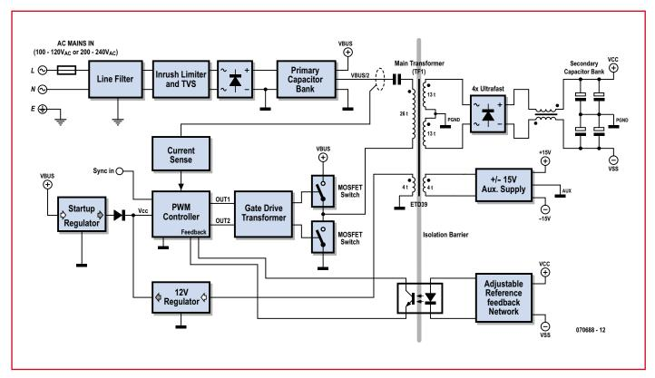
Figuur 1. Block diagram of the SAPS-400. The bulk of work is done by the MOSFETs and transformer TF1; the control goes mainly on account of the PWM controller.
