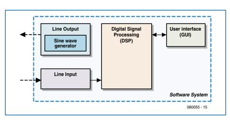
Figure 5. Block diagram of the software.
