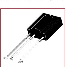
Figure 2. Package and pinout of the TSOP1736.
