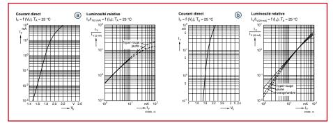
Figure 1. Forward voltage and intensity of a low-current LED (a) and a high-efficiency LED (b).
