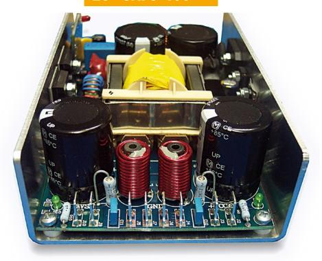
With the SAPS-400 we offer a powerful, adjustable symmetrical supply that's ideal for lightweight audio power amplifiers and happily sits in less than a quarter of the space taken by a comparable supply of conventional design.
