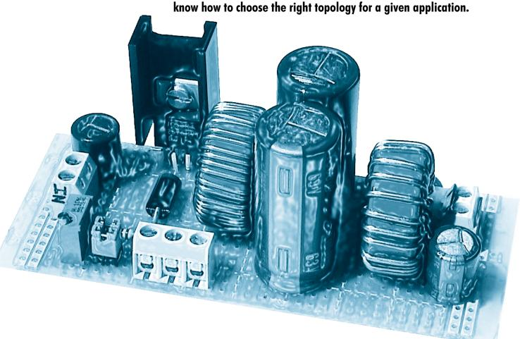
Electronic equipment needs power, mostly in the form of a static voltage (DC). The national grid delivers an alternating voltage (AC), so most electronic devices have a dedicated power supply (PSU) to convert this alternating voltage to the voltage that is needed by the circuitry. This conversion is never 100% efficient.
