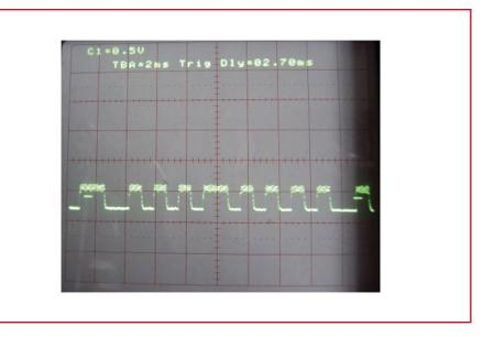
Figure 1. Oscilloscope trace of an RC-5 signal.
