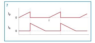
push-pull or half/full-bridges can get at least double the power from the same core volume. But even when a flyback is useful only for <200 W typically, it has lower cost (doesn't need output inductors, uses a single primary switch and secondary diode, etc), and that's one of the main reasons for its popularity. Flyback converters can be found in every TV set, monitors, laptop chargers, small adapters, etc.
