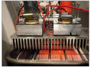
Figure 3. Depke's power generator under test: a gas burner heats from below while cold mineral water flows through the pipe system above. Water condensation results from the coldness and burnt gas.
