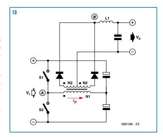
full-bridge converters, on the other hand, allow for a more relaxed rating of the switches, while still providing high output power and good use of the transformer. The schematic of the simpler of both, the half bridge, can be seen in **Figure 10**.
