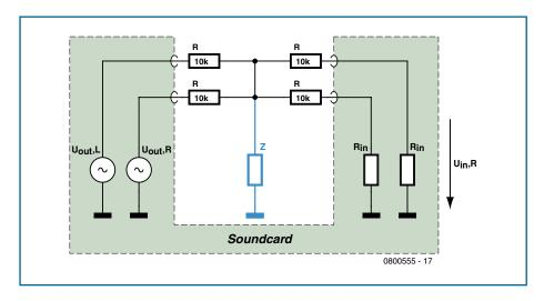
Figure 7. The hardware for method B consists of just four resistors.
