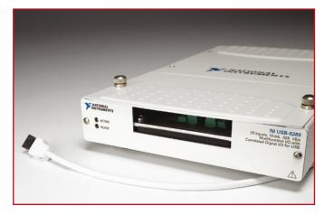
tion to minimise settling time and guarantee maximum accuracy. An onboard lowpass filter can be programmatically enabled to further improve measurement accuracy by eliminating high frequency noise. With the NI USB-628x devices, engineers can deliver an absolute accuracy of 980 µV at a range of ±10 V and 28 µV at a range of
