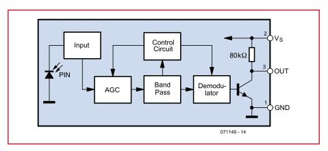
Figure 3. Block diagram of the infrared receiver.
