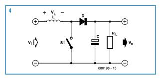
**Figure 4** shows the basic architecture of a boost converter. The analysis is very similar to the buck converter, the main equations being  $V_L = V_i$  (ON state), so:
