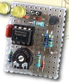
white LEDs this voltage is about  $3.6\ V$ , so at a power supply voltage of  $15\ V$  you can only measure 3 at the same time.
