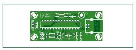
Figure 6. Component mounting plan of the PCB designed for Thermo-Snake. The copper track layout is a free pdf download.
