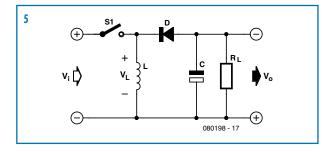
The inverting converter is used to obtain negative voltages from a positive source. **Figure 5** shows the basic schematic. The analysis is very similar to the boost converter. The main equations for the ON state are  $V_L = V_i$ , so:
