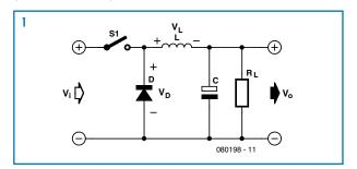
ON (closed), the diode is open as it is directly connected to the input and becomes reverse biased,. Then,  $V_{\rm in}=V_{\rm L}+V_{\rm o}$ , so  $V_{\rm L}=V_{\rm i}-V_{\rm o}$ . The basic equation of an inductor is  $V_{\rm L}=LdI_{\rm L}/dt$ , then
