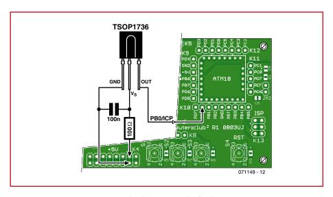
Figure 4. Making the connections to the infrared receiver.
