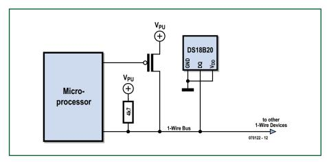
Figure 2. Connecting the DS18B20 temperature sensor on to a 1-Wire network. (courtesy Maxim IC)
