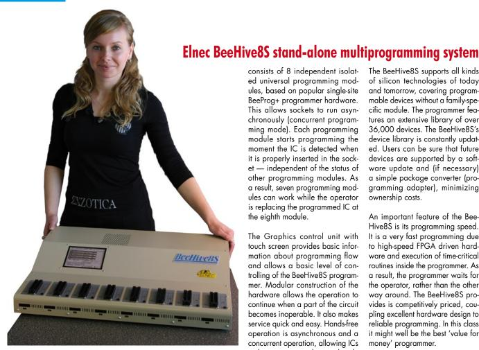
BeeHive8S is an extremely fast universal 8x 48-pindrive Stand-Alone concurrent multiprogramming system designed for high volume pro-
