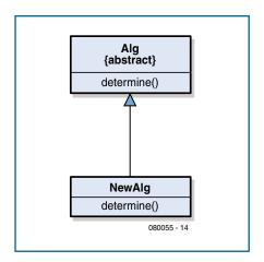
Figure 4. Deriving a new algorithm.
