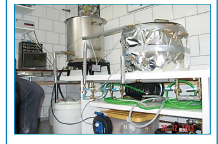
Figure 9. PID controller for brewery.
