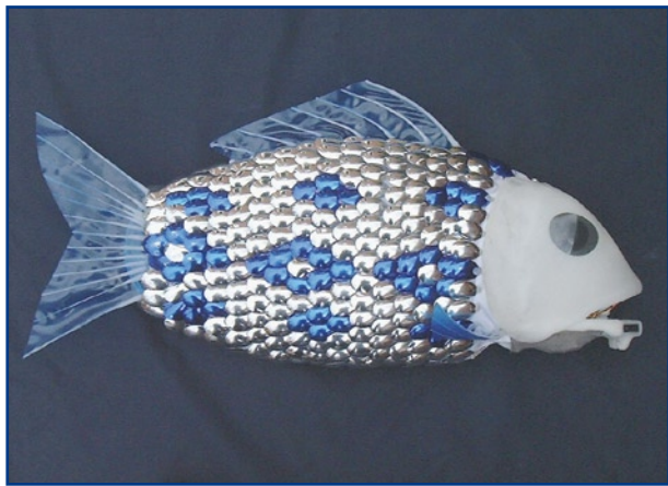
Figure 2. Robot Fish resembles a 50-cm long) common carp, mimics the undulating motions of a real fish swimming and turning. Three Robo-fish swim in a tank in the London aquarium alongside their living counterparts. (courtesy Professor Huosheng Hu, Computer Science Department, Essex University)
