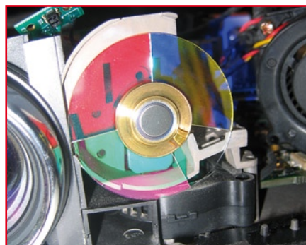
The colour wheel. As can be seen, it consists of red, green and blue segments, plus a white segment for the brightness. At the top right is the position detection PCB.
