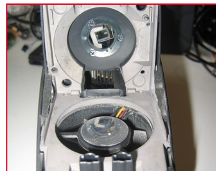
This is where the lamp goes. At the bottom you can see one of the three fans that cool the lamp. The large circular opening goes to the colour wheel and light tunnel.
