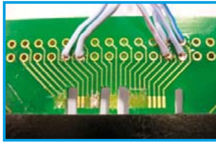
Figure 7. You can also make the matching connector yourself using a PCB designed for SMD components.
