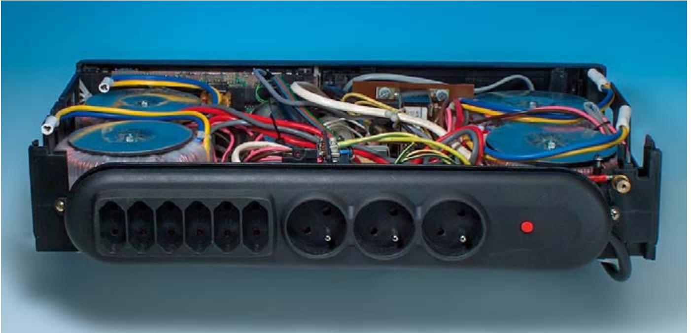
The author connected two transformers in parallel for the prototype, so that they are smaller and the whole filter could fit in a lower enclosure.
