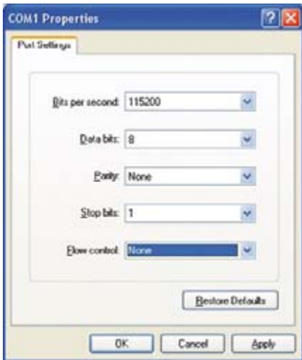
Figure 2. The settings shown here must be used for serial communication.
