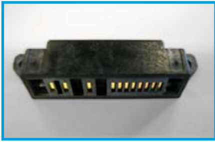
Figure 6. Programming is carried out via this connector on the phone flash. The matching connector illustrated can be bought online.
