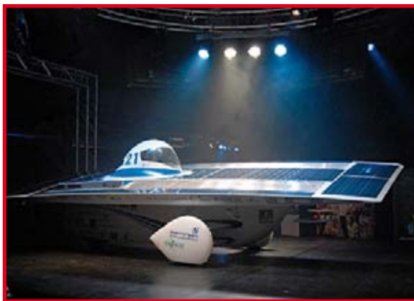
The Twente One with tilting solar panels
