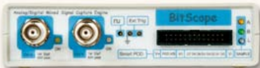
Standard 1M/20pF BNC inputs
