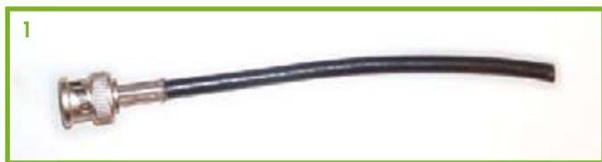
The raw material: a short piece of 50-Ω coax cable.
