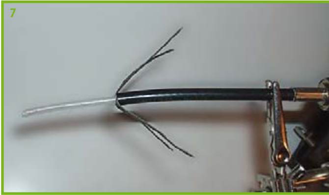
Now bend them into a 45-degree angle with respect to the cable. This angle will result in an antenna impedance of about 50 \Omega .
