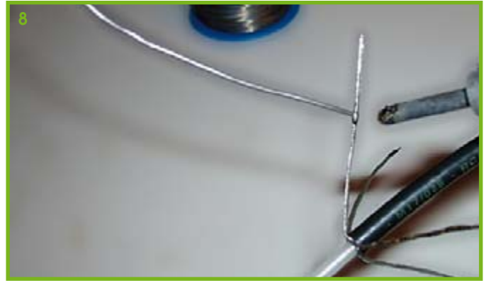
Cover the bundles with solder. Although this step is optional, it does enable the ground plane elements to hold their shape better, and prevents untwisting of the strands.
