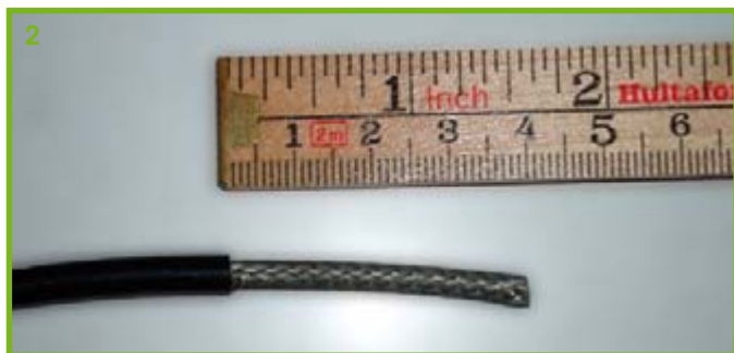
Cut off about 40 mm of the outer insulation. This will expose the braid that forms the cable shield.
