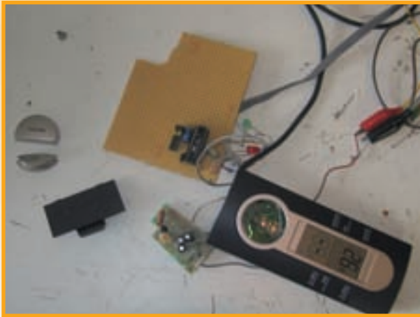
Figure 3. the first prototype of the receiver circuit. On the base station we can see what values the temperature modules are transmitting. Very handy as a check.
