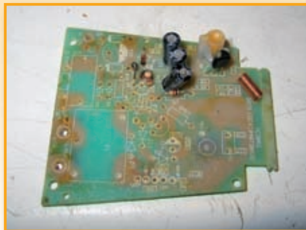
Figure 2. the RF receiver occupies only a small part of the circuit board. These parts (plus the SMD-IC on the other side) are enough to function as an RF receiver.
