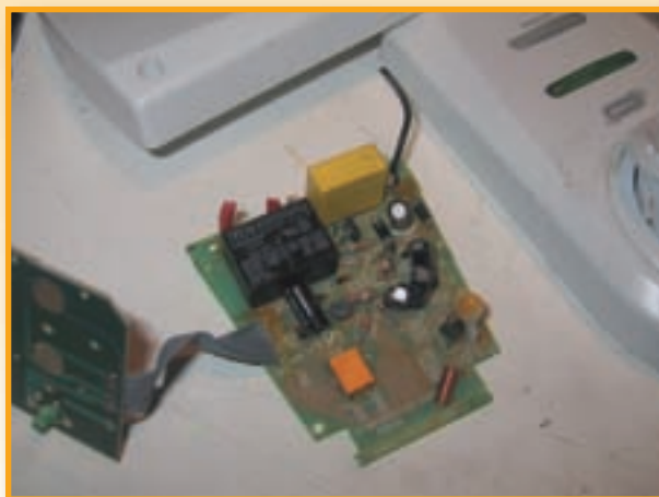
Figure 1. The inside of the remote controlled power point, now still with far too many parts.
