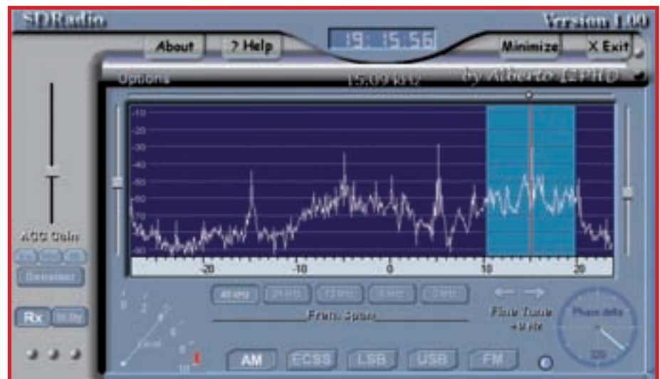
Figure 5. Four AM stations in tuning range spectrum, as displayed by the SDRadio program.
