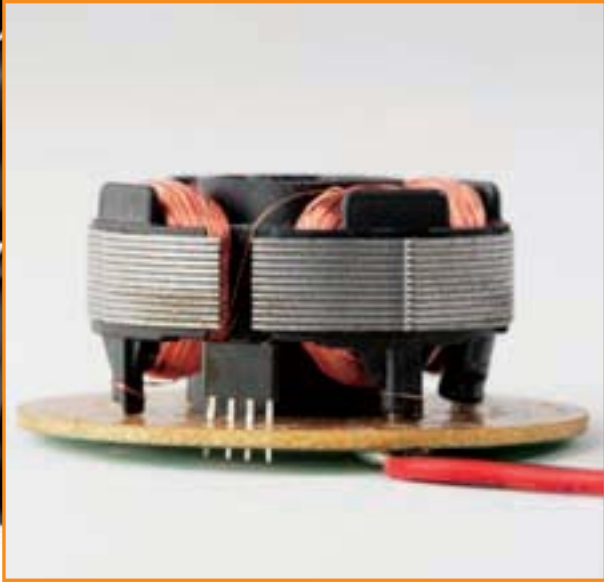
Figure 2. Calling it a rotating magnetic field generator seems to be an overstatement: all the electronics and the Hall sensor are in a 4-pin IC. Apart from an electrolytic capacitor no other components are required.
