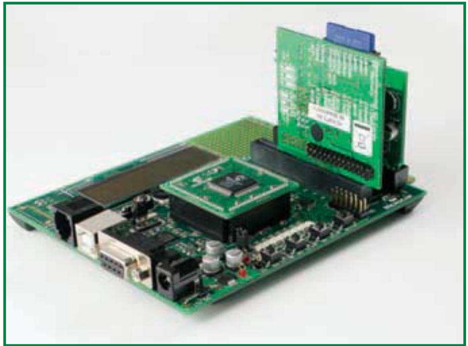
Figure 3. Audio Plus board and CF/MMC board plugged on to the PICtail bus of the Explorer-16 development board.
