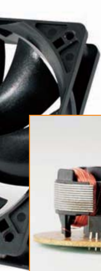
Figure 2. Calling it a rotating magnetic field generator seems to be an overstatement: all the electronics and the Hall sensor are in a 4-pin IC. Apart from an electrolytic capacitor no other components are required.
