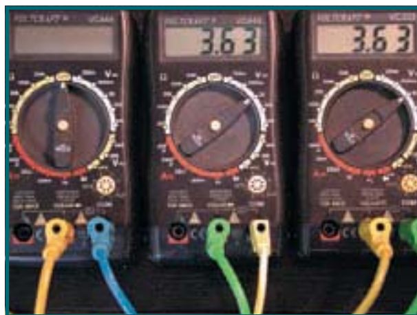
Figure 9. Even a little overcharging does not upset the matching between the two cells of the battery.
