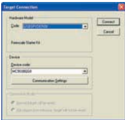
Figure 2. In CodeWarrior, be sure to select the right debugging connection to the PC.
