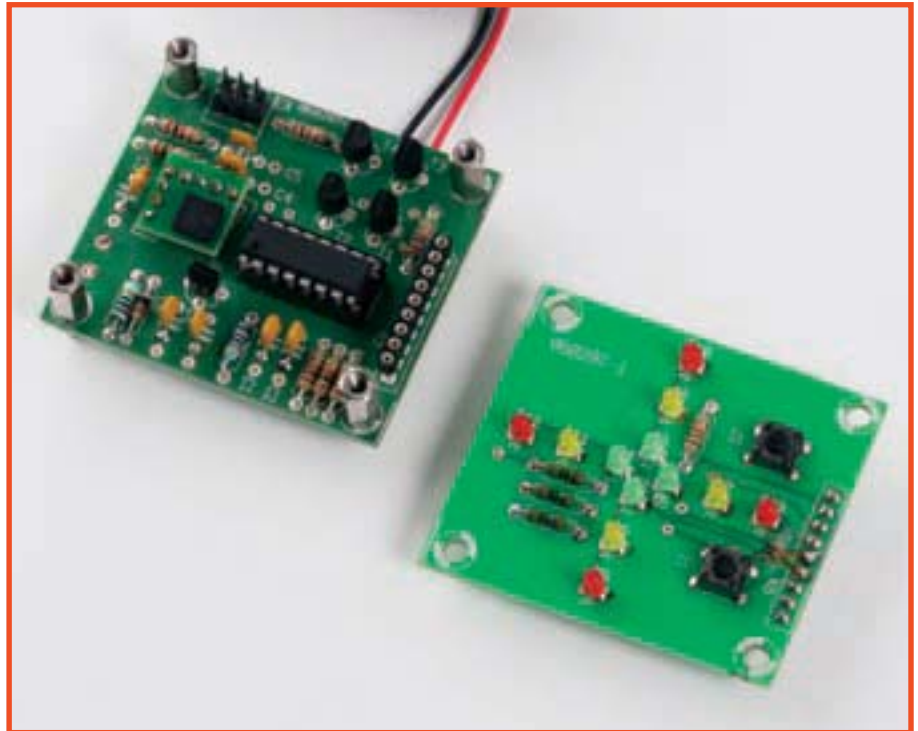
Figure 5. Populated boards prior to assembly with PCB spacers in the four corners.
