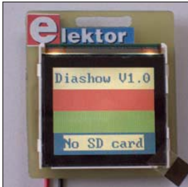
Figure 7. The AVR micro generates a test image when the circuit is turned on for the first time.
