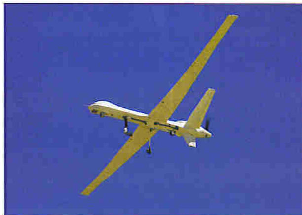
Figure 4. The General Atomics 'Predator' is probably the most recognisable middle category (MALE) drone.
