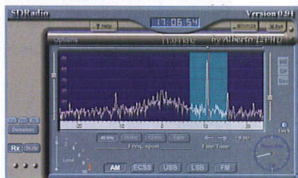
Figure 8. Suppressed image frequency with two mixers.
