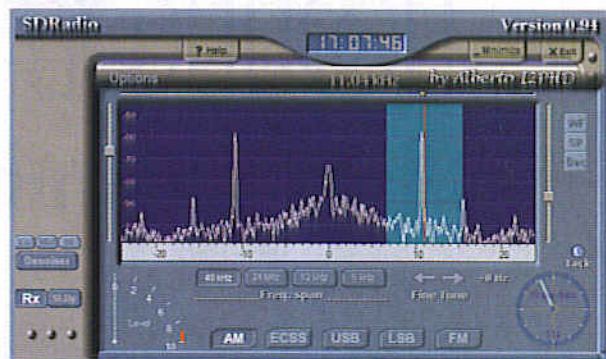
Figure 7. Image frequency with only one mixer.
