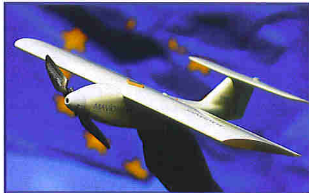
Figure 2. The 'Carolo' is a typical example of a micro UAV using model aircraft components.
