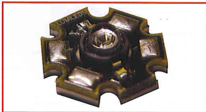
The 'Luxeon III Star Hex' from Lumileds produces up to 80 lm in the white version and up to 190 lm in orange-red. The heatsink has a characteristic six-pointed star shape.
