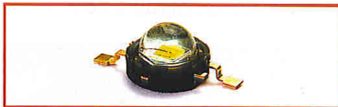
The 'P4' from Seoul Semiconductor is, according to the manufacturer, the brightest LED in the world and can produce more than 240 lm of output at 1 A. At 350 mA the efficiency reaches 100 lm/W. Values of 135 lm/W are expected to be achieved in 2007, and 145 lm/W by the first quarter of 2008.
