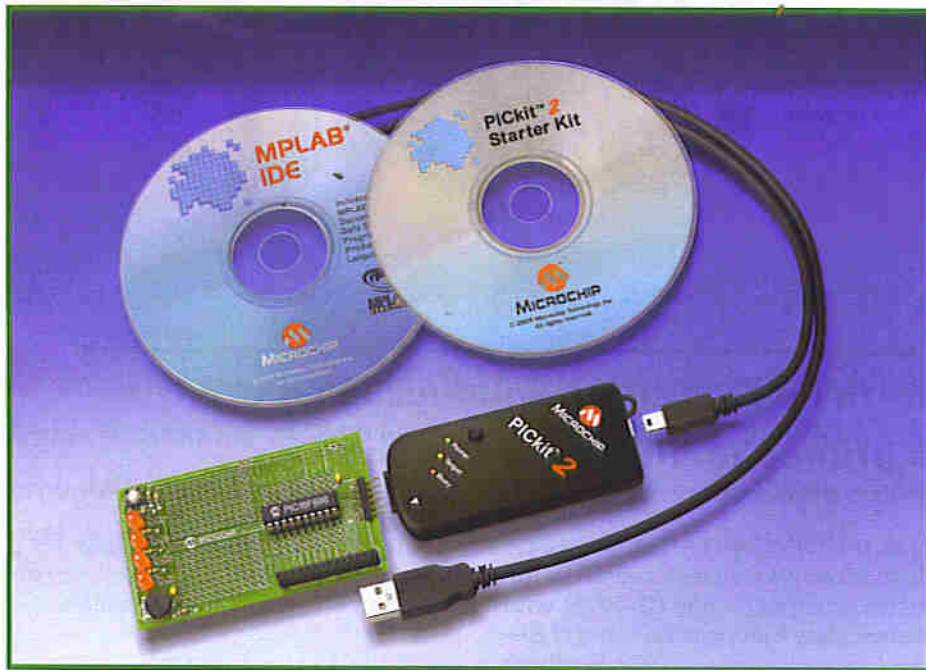
Figure 2. PICkit 2 is a kit-in-a-kit with great potential for all PIC users as it contains a debugger and a programmer.
