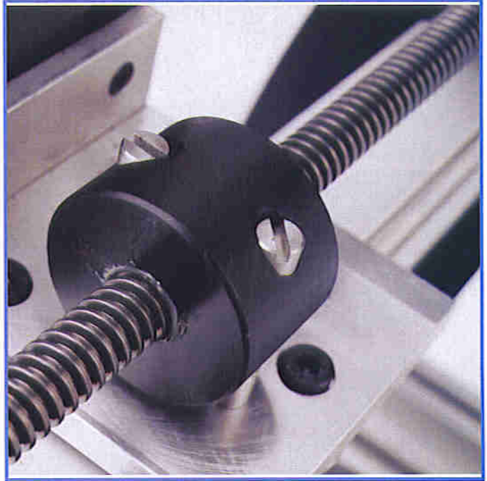
Figure 4. Detail of the plastic nut with the transverse pins, which provide a zero-play coupling.
