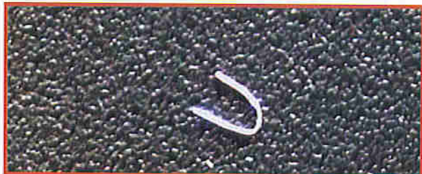
Figure 5. The U shaped wire jumper approximately 2.5 mm long.
