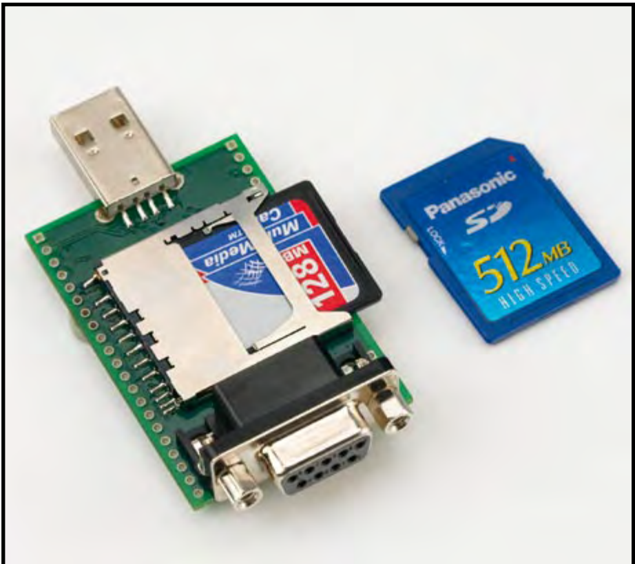
Figure 3. The USB socket, RS232 connector and MMC/SD card holder are the only components mounted on one side of the board.
