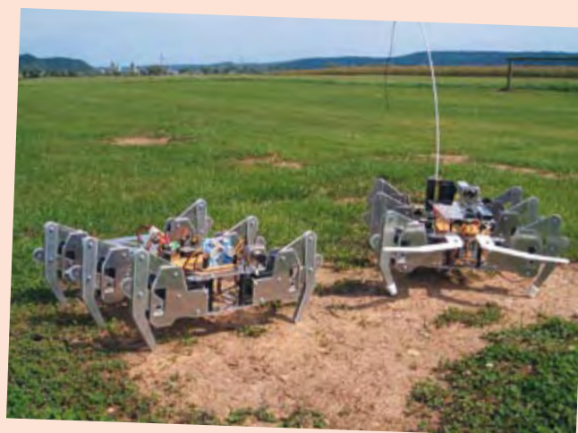
module and the second has an arm that can be raised under servo control to carry a wireless camera. Two additional servos allow this to be moved left and right, also up and down.
