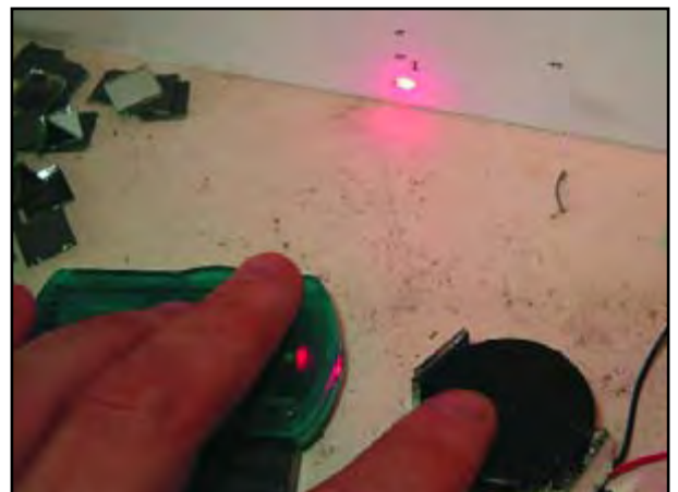
With a sheet of A4 and a laser pointer we can easily set the angle.
