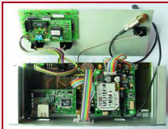
Figure C. Main blocks of the Telematik unit.
