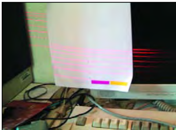
A rotating motor generates lines instead of one concentrated laser dot.
