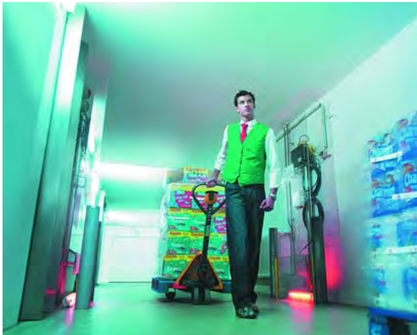
An employee of the Metro trading firm pulls a pallet of diapers through an RFID reader gate, which rapidly reads the data from the chips. The antennas of the RFID reader are located to the left and right (visible on the right side). (photos: Philips)
