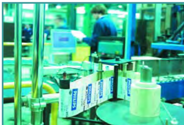
Figure 2. Label inlays on a roll. An inlay consists of a chip, an antenna coil and a substrate (paper or film).
