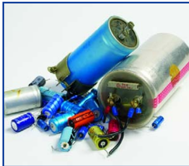
Figure 3. Electrolytic capacitors are a problem for waste disposal. Older types can contain harmful substances such as PCBs.
