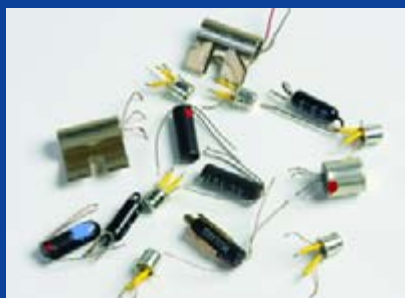
Germanium transistors with their funny AC and OC type codes have a ring of nostalgia around them. A few have been rescued from the landfills. Scratch off the black varnish on some of them and you have a photo sensor.
