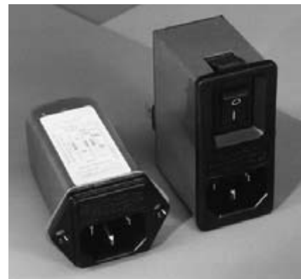
Standard mains filters built into a mains entry together with an on/off switch. The metal shell must be in firm contact with the enclosure.
