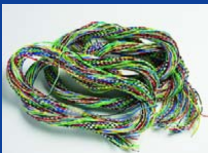
Just a curiosity, this bundle of wires that never made it to the wire loom stage. The individual wires are multi-strand, highly flexible and colour coded. Might reach Flog It status a bit later.
