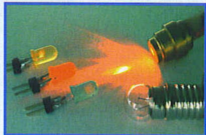
Figure 2. LEDs detecting instead of generating light.
