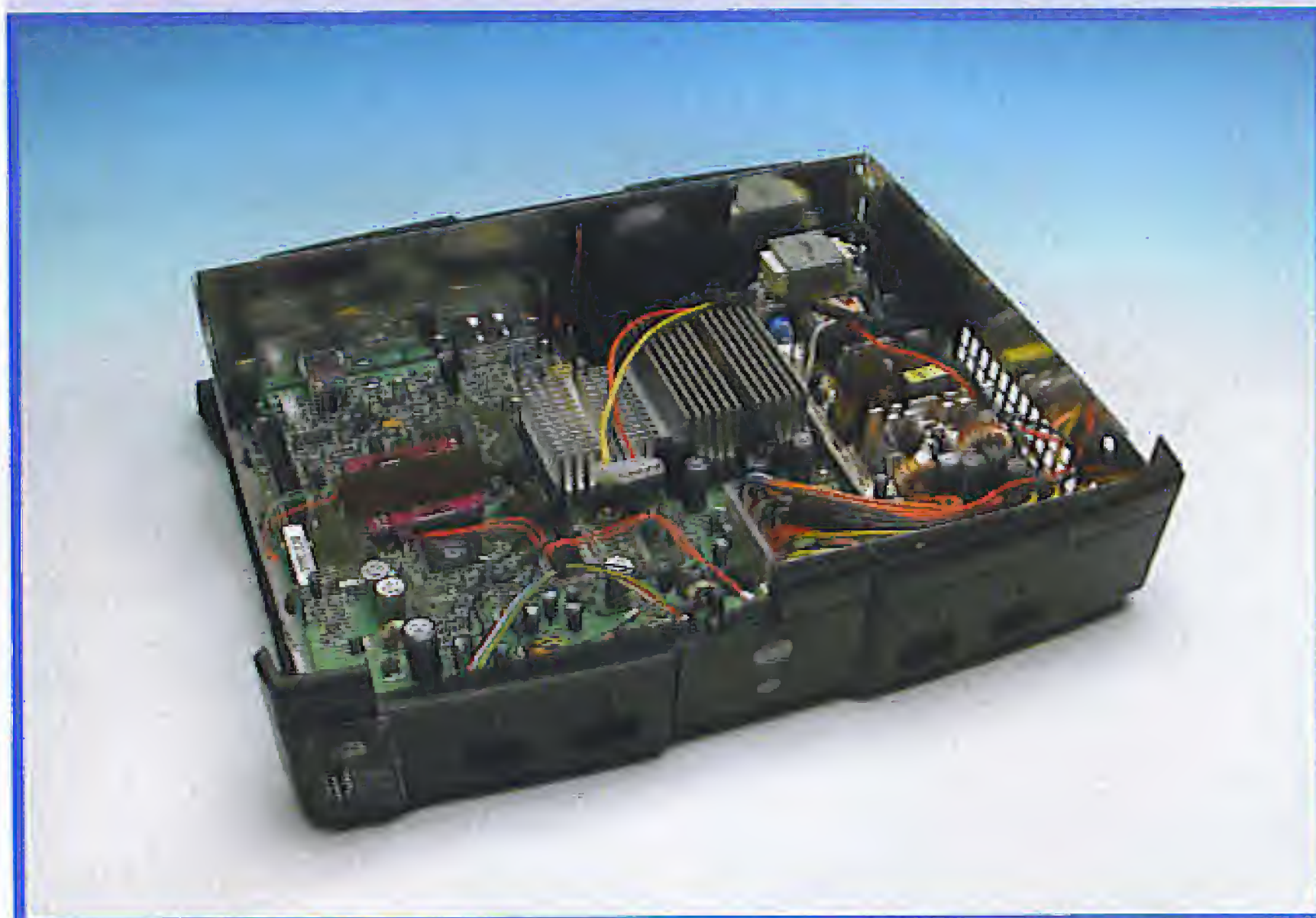
Figure 2. The built-in Xecuter 3 modchip is connected on the left-hand side to a header. At the front on the left-hand side is the accompanying bracket, which is used to install the chip.
