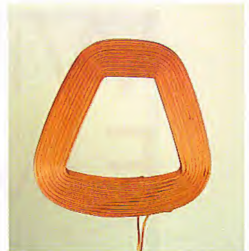
Figure 3. The author's original pick-up coil.
