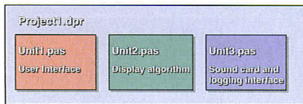
Figure 1. The oscilloscope program is divided into three units.
