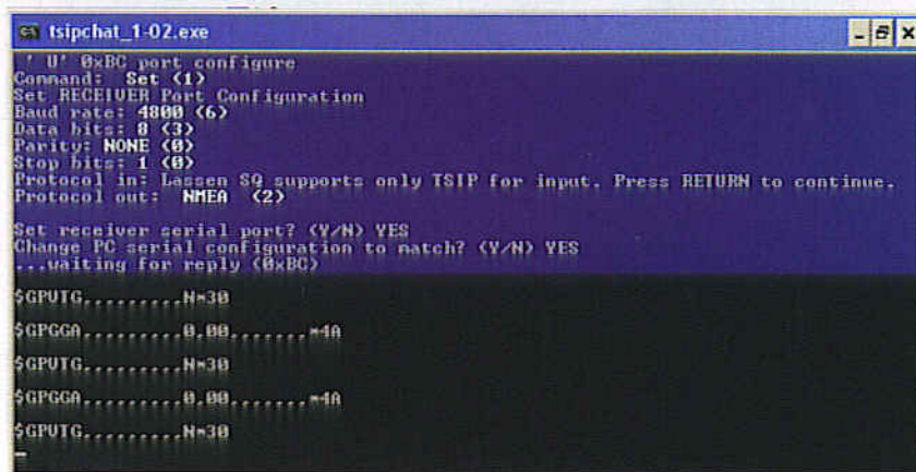
Figure 6. Interface configuration using the 'TSIPChat' program.
