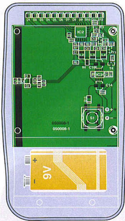
FIGURE 3. Copper track layout and component mounting plan of the PCB designed for the tester. The dipole antenna is a stripline circuit.
