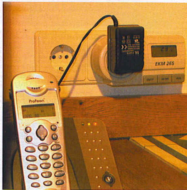
Figure 1. Power measurements are easy — just insert the instrument between the power outlet and the plug. You'll be surprised about the results of the test!
