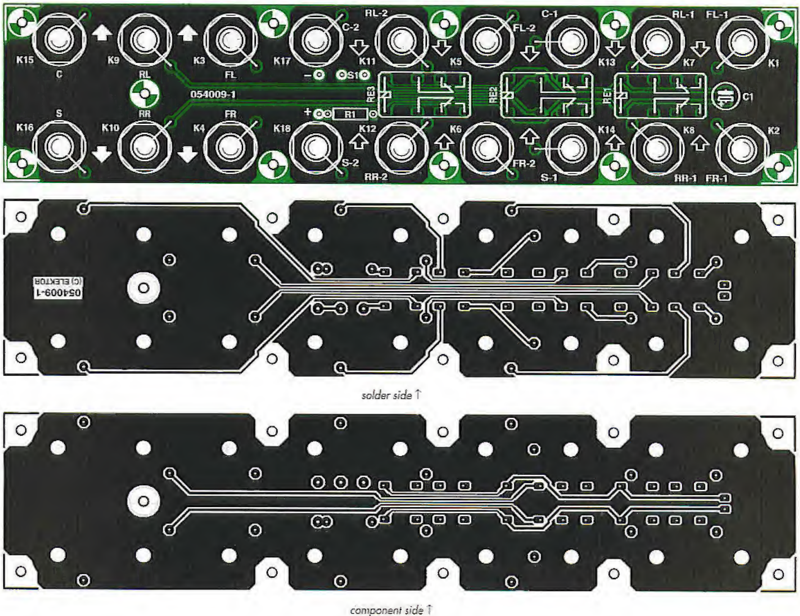
Figure 2. The PCB has been designed for maximum channel separation (note the earth plane running between signal lines).
