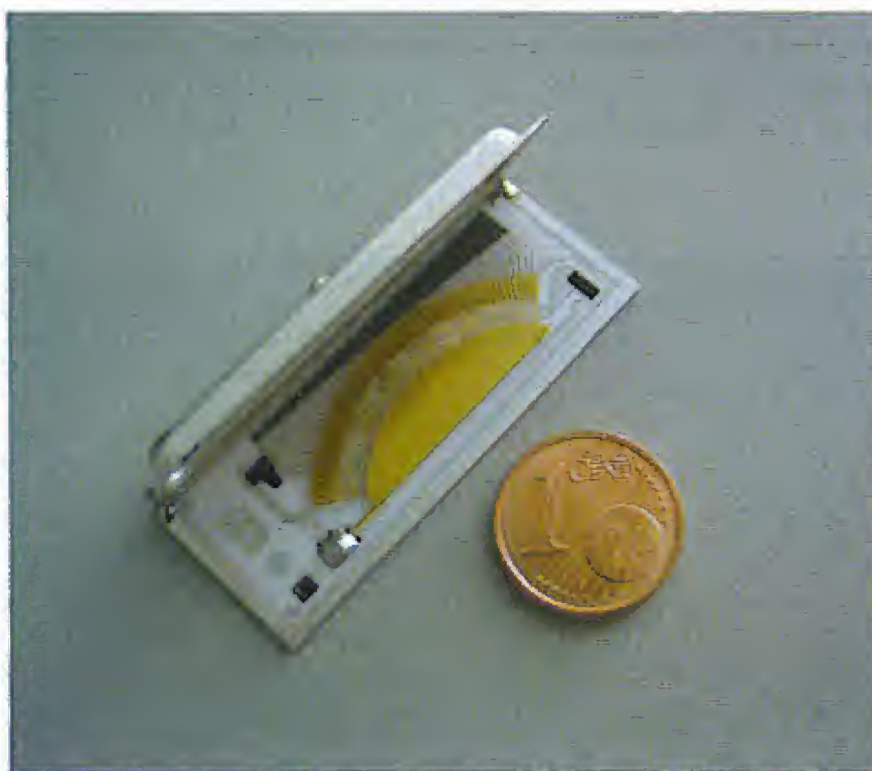
Figure 5. A high-reliability fuel level sensor with many fine contact arms actuated by an external magnet passing alongside the contacts. (Source: Siemens-VDO)
