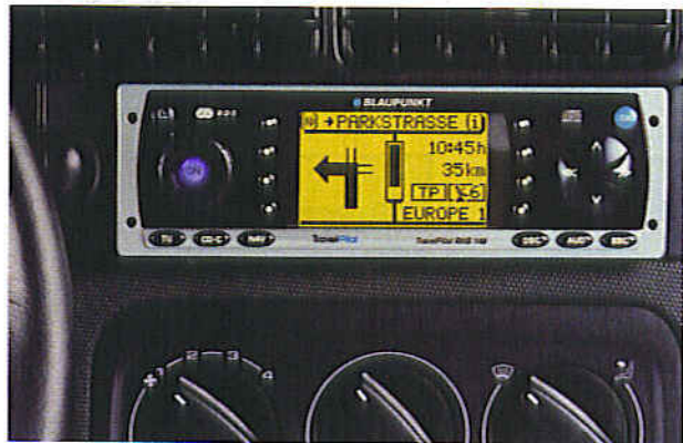
Figure 1. The TravelPilot RNS 149 from Blaupunkt crams a car radio, CD player and navigation system into a standard DIN vehicle radio-housing format. (photo: Blaupunkt)
