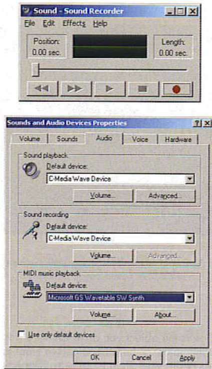
Figure 4. The Windows Sound Recorder makes it easy to record a signal via the sound card.
