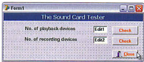
Figure 5. This test program detects which sound options are present in the PC.
