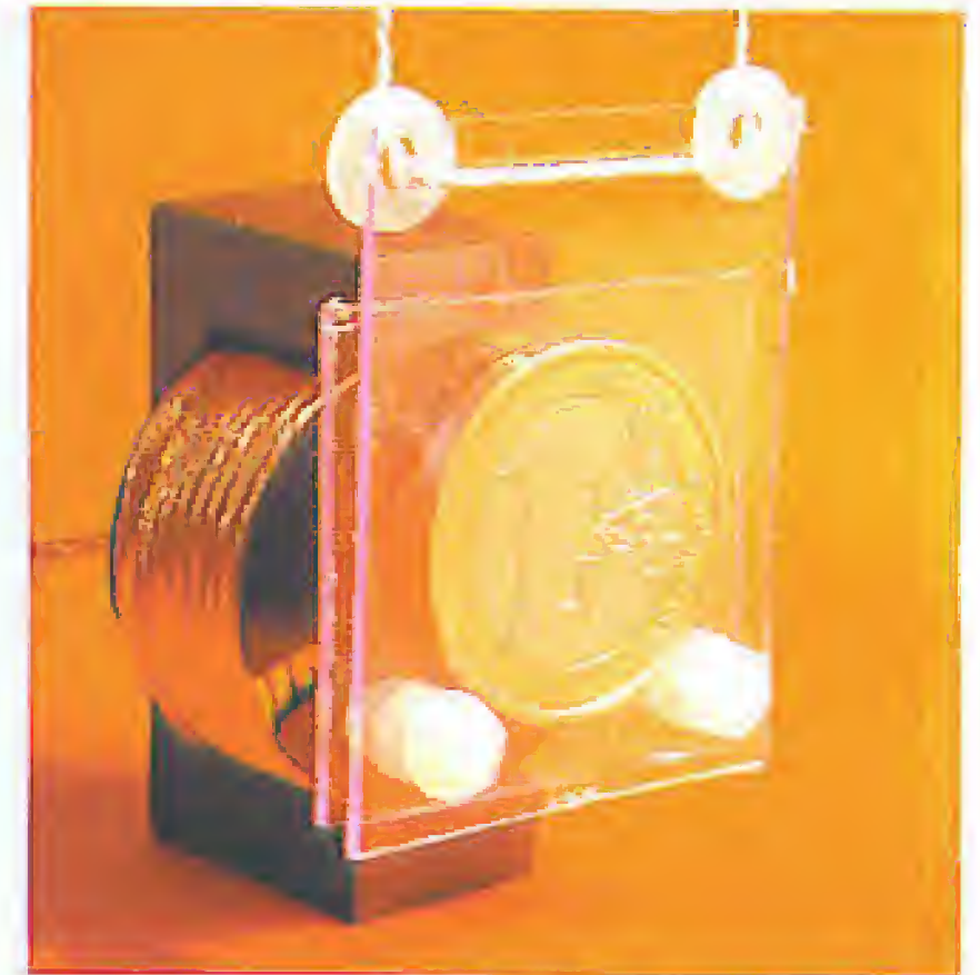
A one-euro coin freely suspended in front of an electromagnet.
