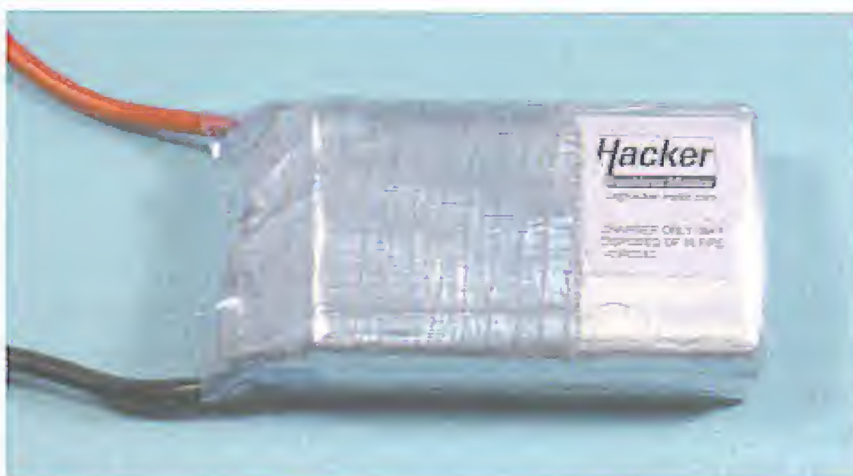
Figure 8. A wide piece of tape serves as a strain relief for the connection wires.
