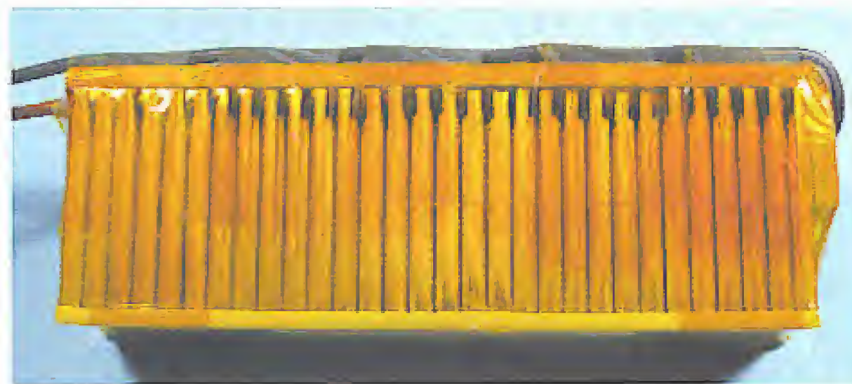
Figure 9. Hand-made Li-polymer battery using thirty 850 mAh cells in a 5S6P configuration. The 5.1 Ah, 18.5 V pack can deliver currents up to 10 C (51 A).
