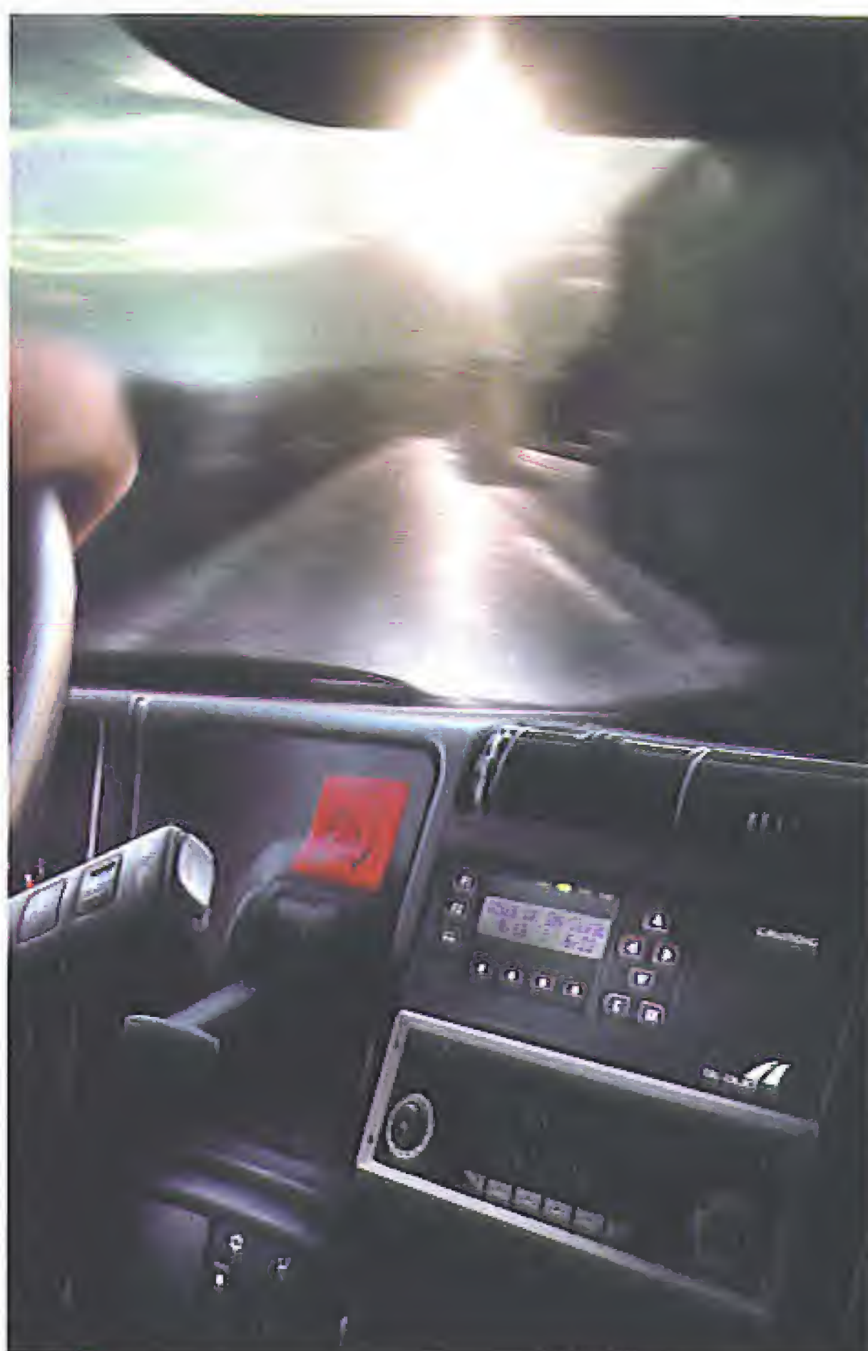
Figure 1. The dash-mounted On-Board Unit (OBU) automatically logs motorway toll sections. The driver can input vehicle configuration variables (e.g. the lorry may be travelling without a trailer). (Picture: Grundig)
