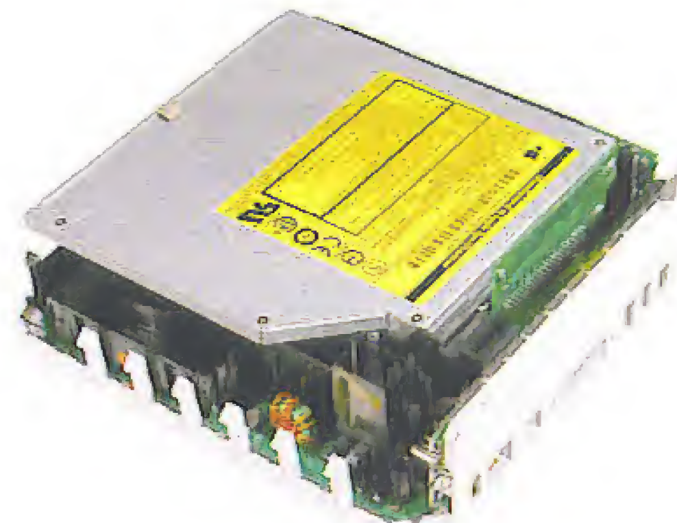
Figure 3. Inside the Mac Mini. At the top is the ultra-slim optical drive, behind which hides the 2.5" hard disk. Below, to the left, part of the centrifugal black CPU fan can be seen. Above and to the right is the main memory: a standard PC2700 DDR DIMM with 184 pins.
