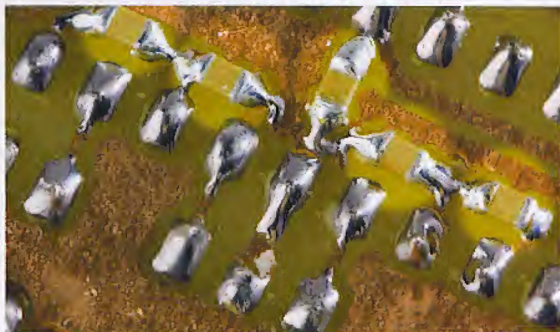
Figure 4. Some components need to be fitted at the solder side of the board, too.
