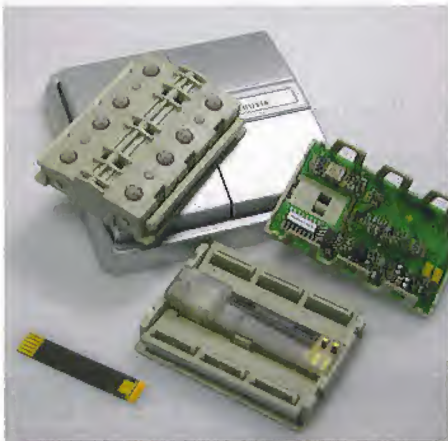
Figure 1. The battery-free piezo transmitter module PTM 100 (on the switch plate). Individual components are seen in the foreground: Piezo converter (left), mechanical energy converter, and PCB with Antenna. (source: EnOcean GmbH)
